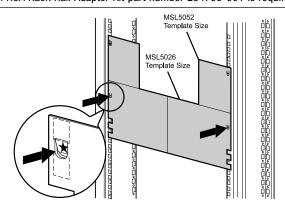
Use the template shipped with the library to mark the location of the mounting hardware on the mounting rails of the storage cabinet.
