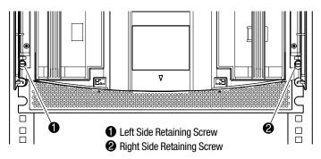
With the doors open, secure the front panel to the storage cabinet using the two retaining screws. Close the doors before proceeding to Step 5.
