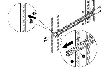
e. Remove the template, then attach the rails using the supplied fasteners. Rail front brackets are threaded to directly accept screws. Rear brackets are not threaded and require installation of cage nuts in the storage cabinet's rear vertical rails. Refer to the Compaq Rack Products Reference Guide for detailed cage nut installation instructions.
