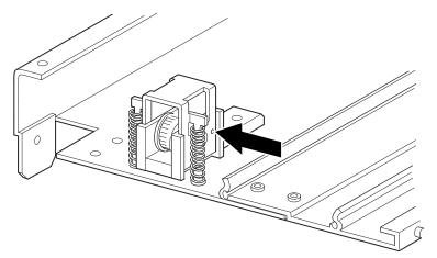
Figure 19: Tensioner ramp/idler pulley zero point
