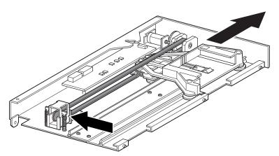
Figure 14: Media elevator car location
