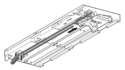
Figure 21: Installing the timing belt
