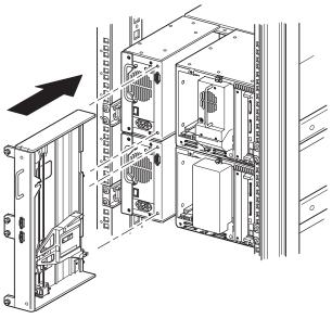
Figure 9: Installing the PTM base unit
