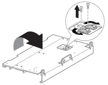
Figure 15: Belt block bracket access cutout
