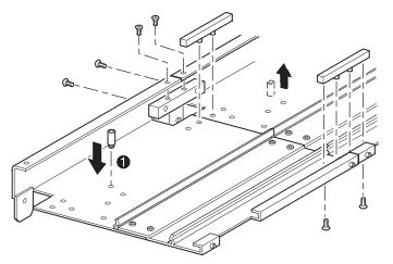
Figure 18: Installing tie bars
