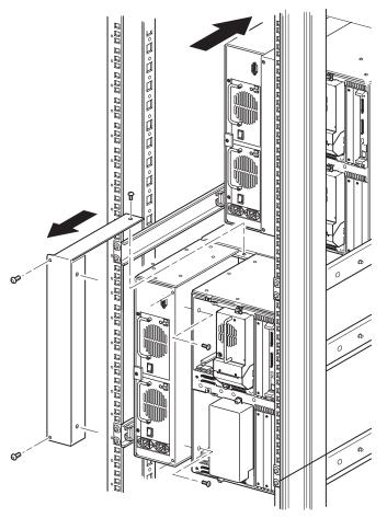
Figure 12: Removing a PTM cover plate (10U models)
