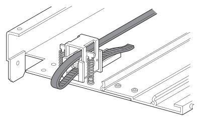
Figure 20: Installing the timing belt on the extension
