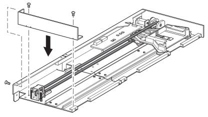
Figure 23: Installing the bottom plate
