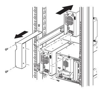
Figure 8: Removing the PTM cover plate
