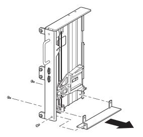
Figure 13: Removing the bottom plate from the PTM base unit
