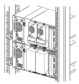
Figure 6: 5U library installation (9000 rack enclosure shown)
