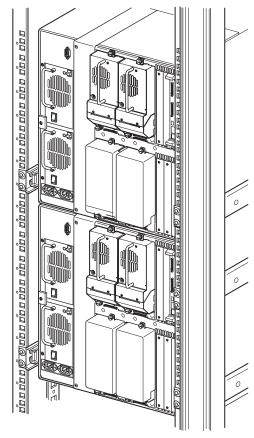
Figure 10: Library installation, 10U models (9000 rack enclosure shown)
