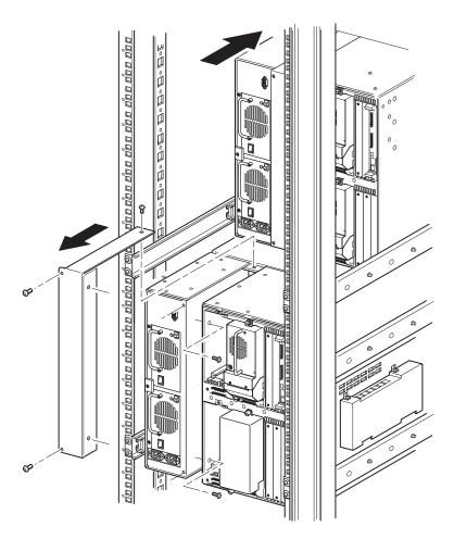
Figure 2–9: Removing a PTM cover plate (MSL5052)
