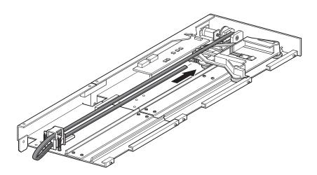
Figure 2–18: Installing the timing belt
