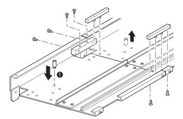
Figure 2-15: Installing tie bars
