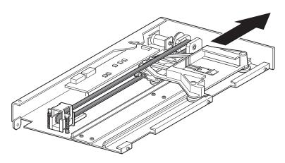
Figure 2–11: Media elevator car location
