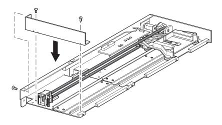
Figure 2–20: Installing the bottom plate
