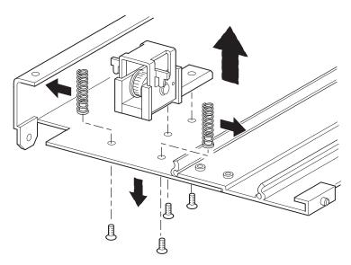
Figure 2–13: Removing the belt tensioner ramp and idler pulley
