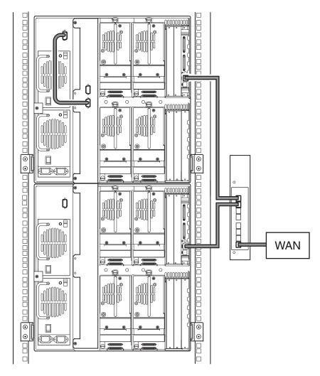
Figure 2–21: MSL5052 multi-unit library configuration (single master and slave)
