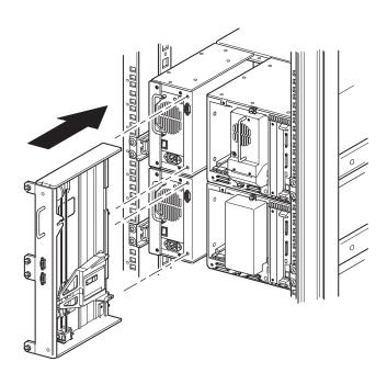
Figure 2-6: Installing the PTM base unit
