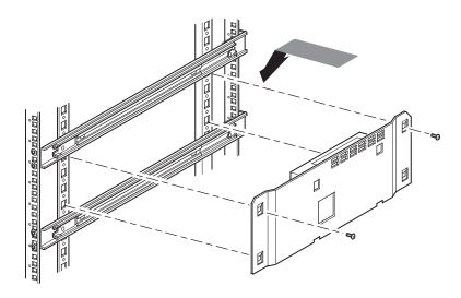
Figure 2-1: Installing the router into a Compaq storage cabinet
