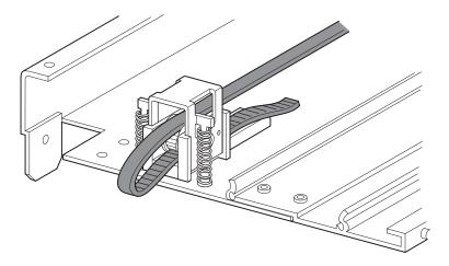
Figure 2–17: Installing the timing belt on the extension
