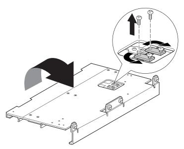
Figure 2-12: Belt block bracket access cutout
