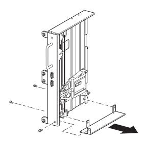
Figure 2-10: Removing the bottom plate from the PTM base unit
