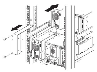
Figure 2-5: Removing the PTM cover plate
