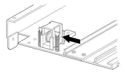
Figure 2-16: Tensioner ramp/idler pulley zero point
