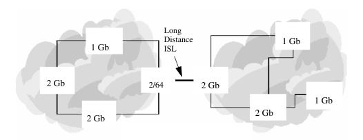
Figure 3: Mixed Extended Fabric with Core Switch 2/64 to StorageWorks 2 Gb SAN switch ISL long distance port switches
