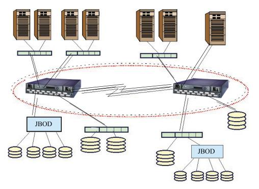
Figure 3: QuickLoop configured as long-distance QuickLoop
