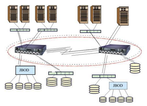
Figure 2: QuickLoop configured as dual-switch
