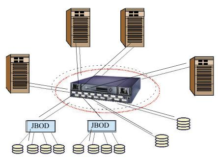
Figure 1: QuickLoop-enabled switch used as concentrator
