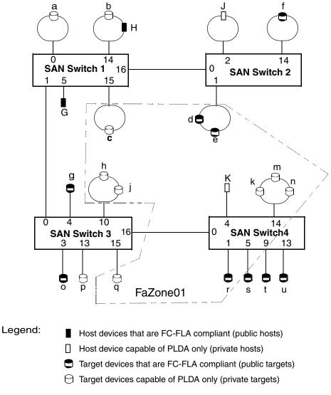
Figure 2: Fabric Assist Mode Zone Configuration Example
