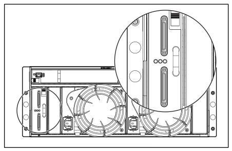
Figure 4-5: SCSI I/O board connectors
