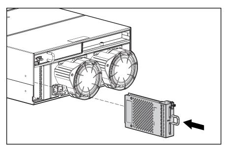
Figure 2-20: Installing the I/O EMU
