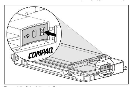
Figure 4-9: Drive failure indicator
