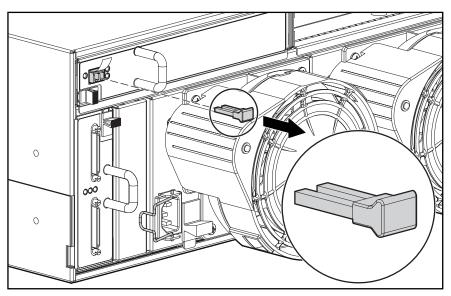
Figure 2-24: Removing the dust cover from the SFP
