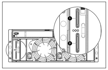
Figure 2-27: MSA 1000 expansion SCSI connectors
