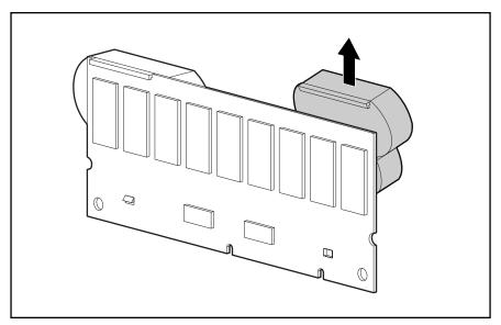
Figure 2-12: Removing the battery pack
