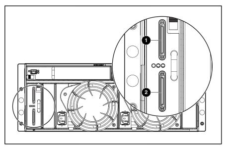
Figure 2-28: MSA 1000 expansion SCSI connectors
