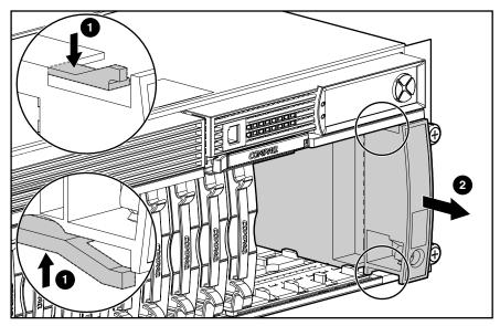
Figure 2-32: Removing the power switch assembly
