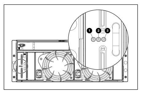
Figure 4-10: SCSI I/O Module with Integrated Environmental Monitoring Unit (I/O EMU)
