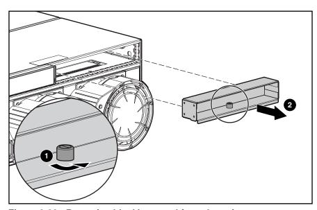
Figure 2-29: Removing blanking panel from the unit
