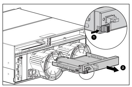
Figure 2-21: Removing the MSA 1000 Fibre Channel I/O module
