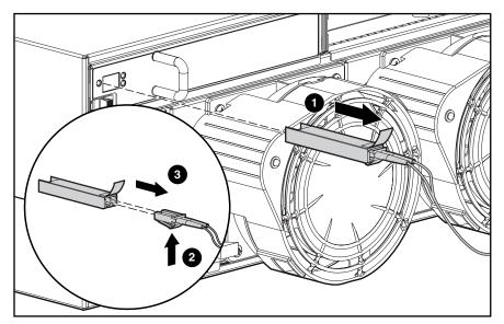
Figure 2-22: Removing the failed SFP
