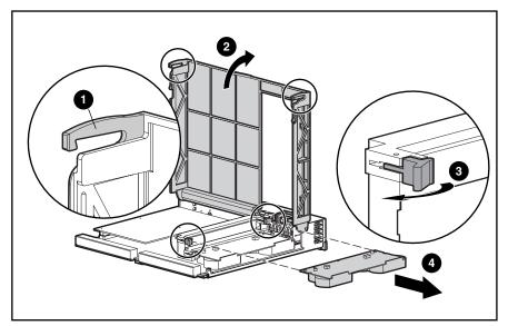
Figure 2-8: Replacing the cache module
