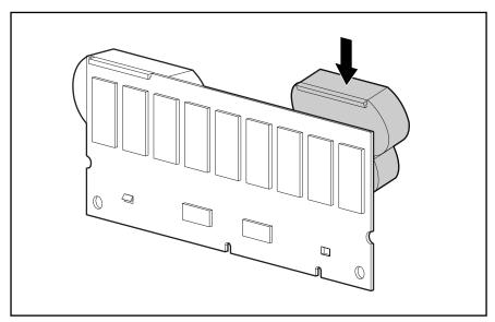
Figure 2-13: Installing the battery pack
