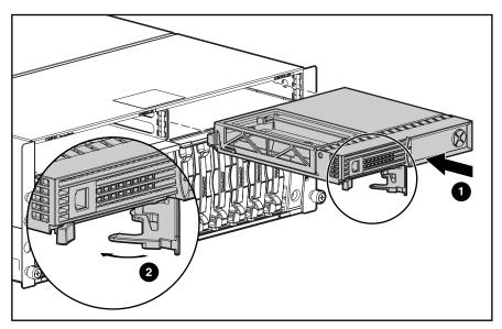
Figure 2-6: Installing the replacement controller
