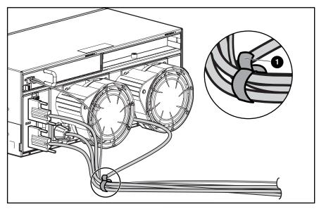
Figure 2-26: Cable management using cable ties
