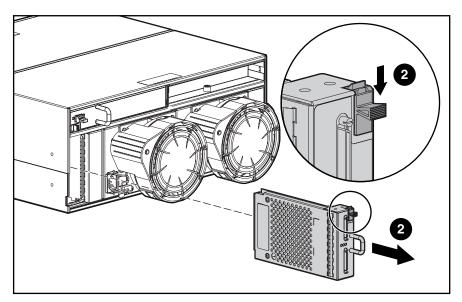
Figure 2-19: Removing the MSA 1000 I/O EMU
