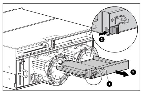
Figure 2-30: Removing the Fibre Channel I/O module
