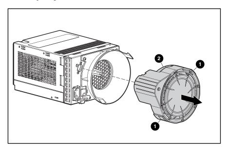
Figure 2-15: Removing the blower
