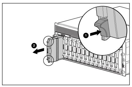
Figure 2-1: Removing an MSA 1000 hard drive blank
