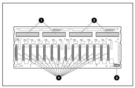
Figure 4-3: Backplane board front connectors: controller connectors ①, controller connectors ②, power switch connector ③, hard drive connectors ④
