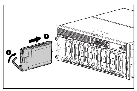
Figure 2-4: Inserting the new drive
