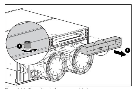
Figure 2-34: Removing the interconnect blank
