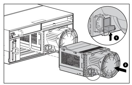
Figure 2-18: Installing the replacement power supply
