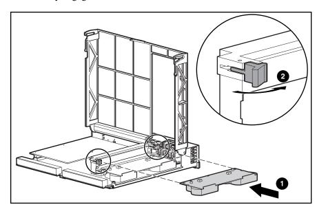
Figure 2-9: Installing the cache module
