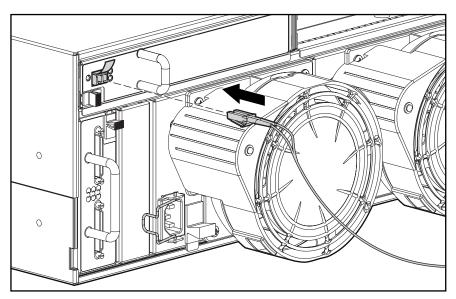
Figure 2-25: Installing the Fibre Channel I/O cable
