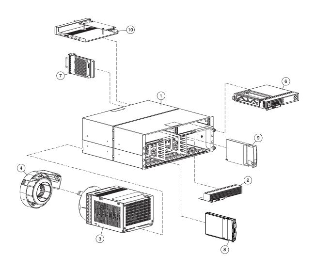
Figure 1-1: MSA 1000 mechanical parts and system components exploded view
