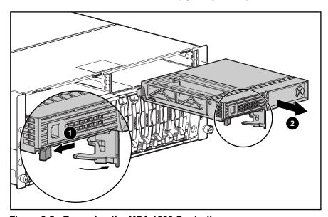
Figure 2-5: Removing the MSA 1000 Controller
