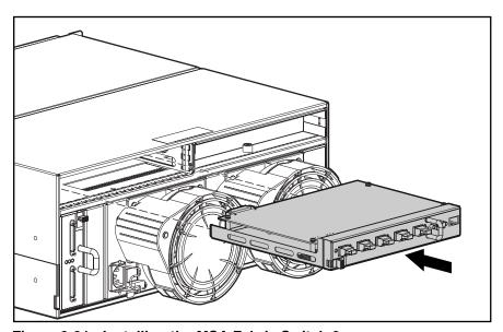
Figure 2-31: Installing the MSA Fabric Switch 6
