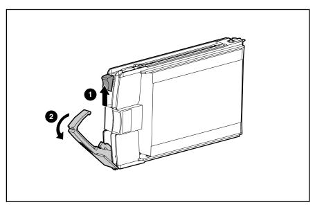
Figure 2-3: Pressing the ejector and pulling the lever
