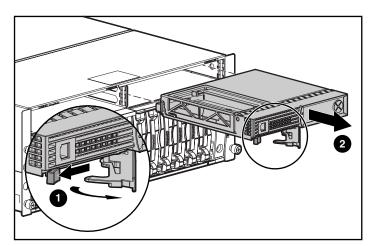
Figure 2-7: Removing the controller
