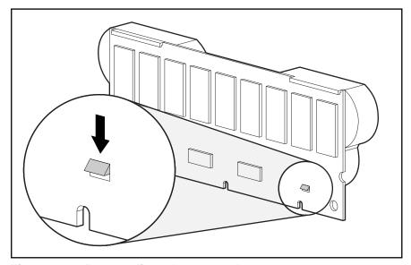
Figure 2-10: Bottom clip on battery pack
