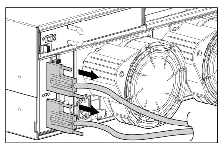
Figure 2-36: Removing SCSI cables
