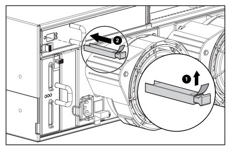
Figure 2-23: Installing a new SFP
