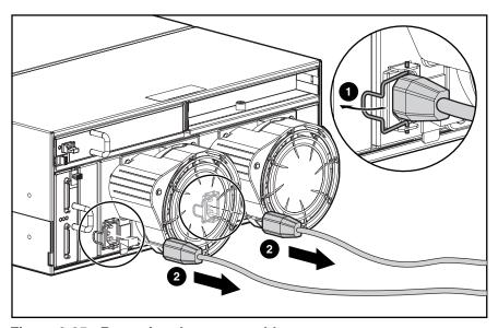
Figure 2-35: Removing the power cables
