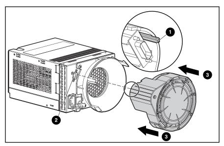
Figure 2-16: Installing the replacement blower
