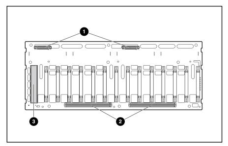
Figure 4-4: Backplane board back connectors: Fibre Channel connectors **①**, power supply connectors **②**, I/O EMU connector **③**
