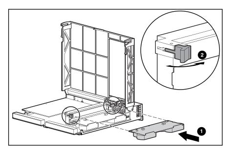
Figure 10: Installing the cache module
