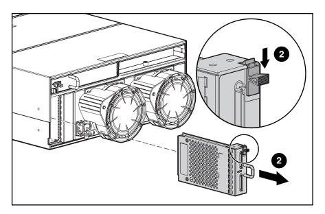
Figure 20: Removing the MSA1000 I/O EMU
