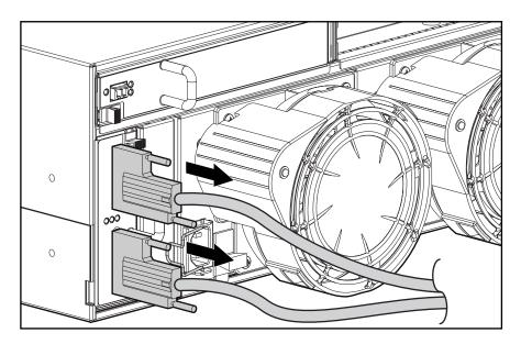
Figure 37: Removing SCSI cables
