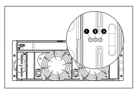
Figure 48: SCSI I/O Module with Integrated Environmental Monitoring Unit (I/O EMU)
