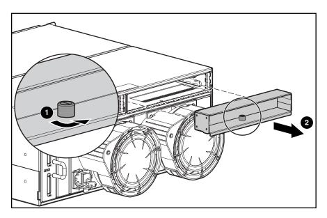
Figure 35: Removing the interconnect blank
