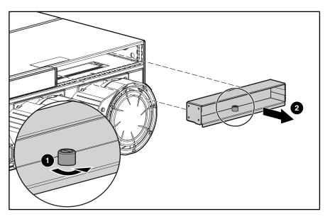
Figure 30: Removing blanking panel from the unit
