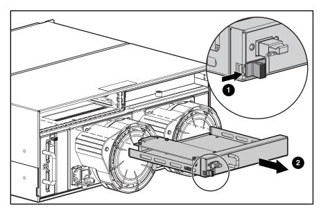
Figure 22: Removing the MSA1000 Fibre Channel I/O module
