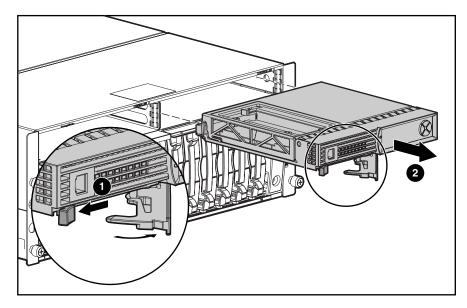
Figure 6: Removing the MSA1000 Controller
