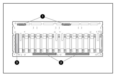
Figure 42: Backplane board back connectors: Fibre Channel connectors  $\mathbf{0}$ , power supply connectors  $\mathbf{0}$ , I/O EMU connector  $\mathbf{0}$
