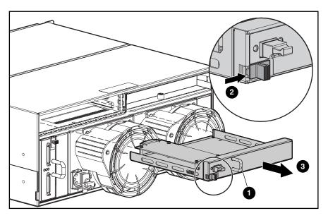
Figure 31: Removing the Fibre Channel I/O module
