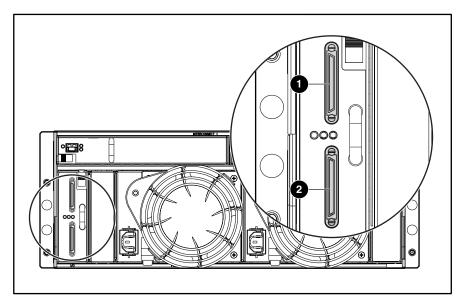
Figure 28: MSA1000 expansion SCSI connectors
