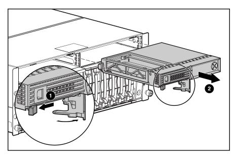
Figure 8: Removing the controller
