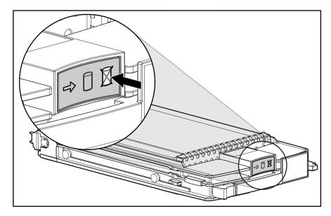
Figure 47: Drive failure indicator
