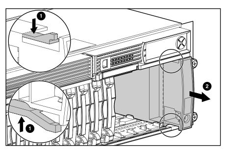
Figure 33: Removing the power switch assembly
