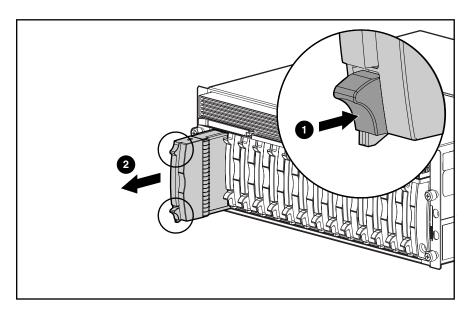
Figure 2: Removing an MSA1000 hard drive blank
