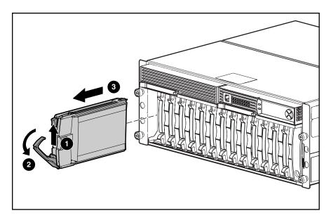
Figure 3: Removing an MSA1000 hot-plug hard drive
