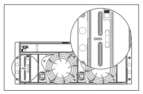
Figure 43: SCSI I/O board connectors
