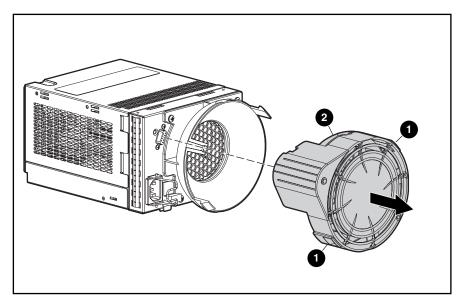
Figure 16: Removing the blower
