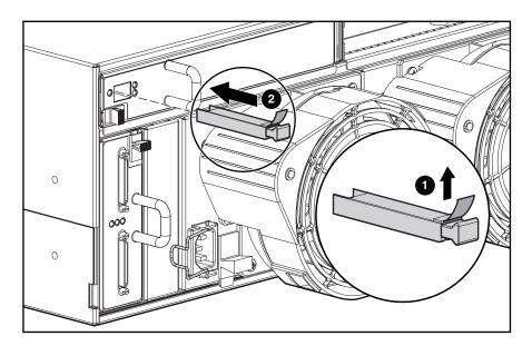
Figure 24: Installing a new SFP
