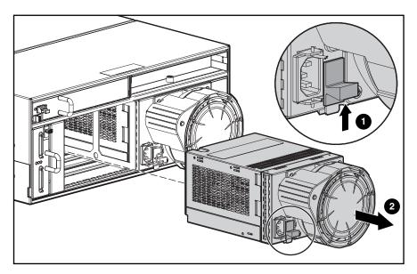
Figure 18: Removing the power supply
