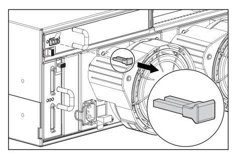
Figure 25: Removing the dust cover from the SFP
