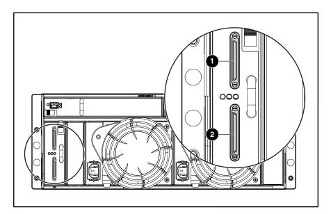
Figure 29: MSA1000 expansion SCSI connectors
