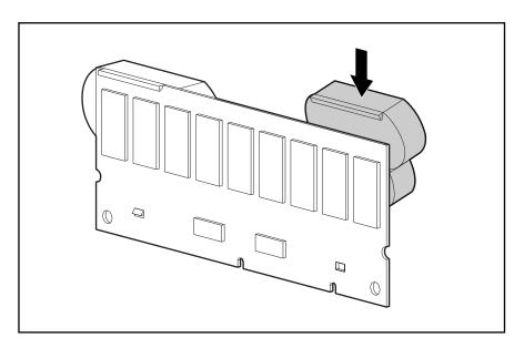
Figure 14: Installing the battery pack
