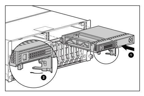
Figure 7: Installing the replacement controller
