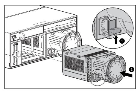
Figure 19: Installing the replacement power supply
