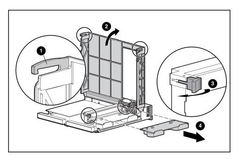
Figure 9: Replacing the cache module
