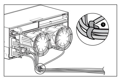
Figure 27: Cable management using cable ties
