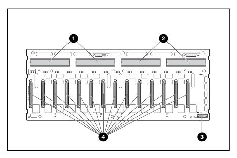
Figure 41: Backplane board front connectors: controller connectors **3**, controller connectors **4**, power switch connector **4**, hard drive connectors **4**
