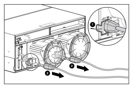
Figure 36: Removing the power cables
