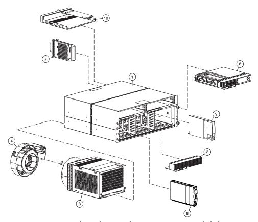
Figure 1: MSA1000 mechanical parts and system components exploded view
