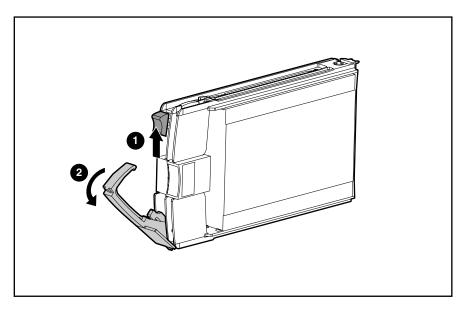
Figure 4: Pressing the ejector and pulling the lever
