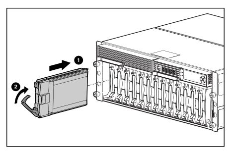
Figure 5: Inserting the new drive
