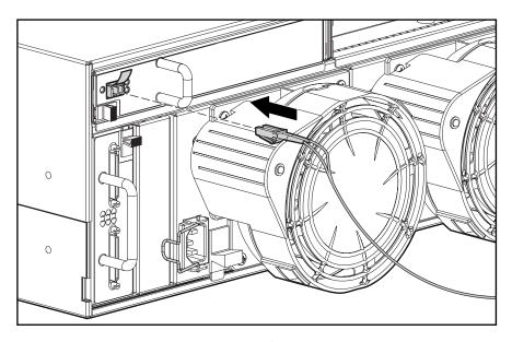
Figure 26: Installing the Fibre Channel I/O cable
