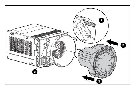
Figure 17: Installing the replacement blower
