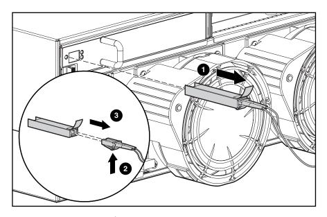
Figure 23: Removing the failed SFP
