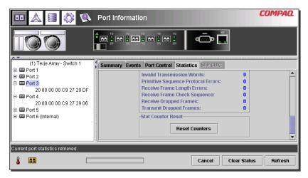
Figure 31: Stat counter reset view
