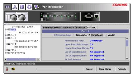
Figure 34: SFP tab – operational display
