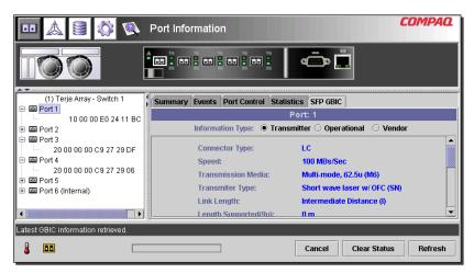
Figure 32: SFP tab - transmitter display
