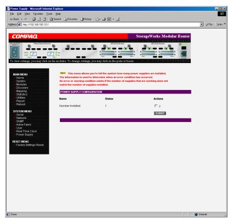
Figure 4-13: Power supply screen
