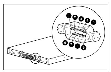
Figure A-1: DB-9 Serial pin assignments
