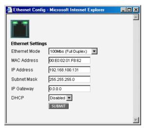
Figure 4-8: Ethernet Configuration dialog box
