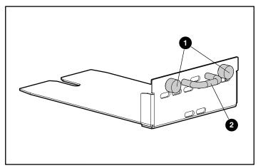
Figure 7-7: Thumbscrews and handle on an I/O module or blank module
