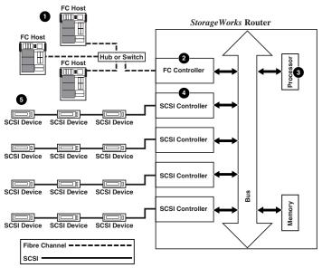
Figure 1-10: Converting Fibre Channel to SCSI process
