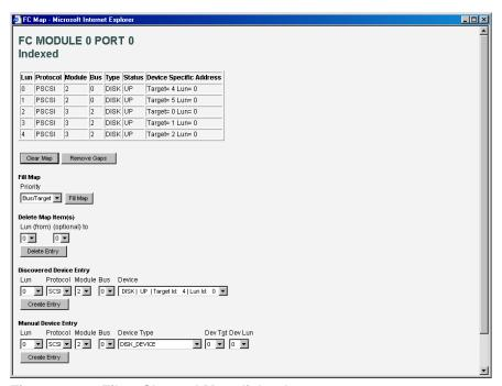
Figure 4-28: Fibre Channel Map dialog box
