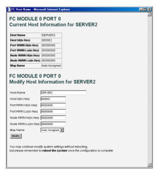
Figure 4-27: Fibre Channel Host Name dialog box
