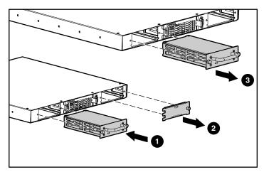
Figure 7-1: Removing and installing power modules
