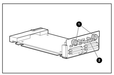
Figure 7-8: Thumbscrews and handle on a SCSI module
