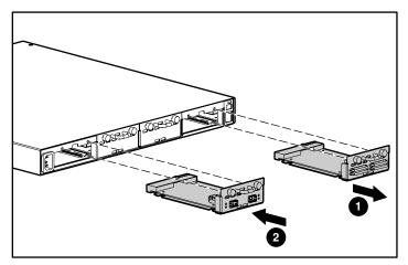
Figure 7-6: Removing and installing I/O modules
