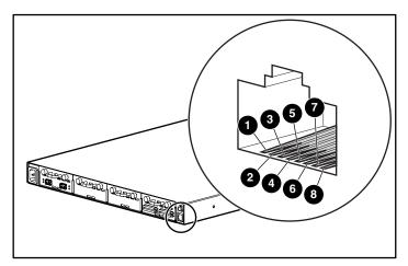
Figure A-2: RJ-45 Ethernet pin assignments
