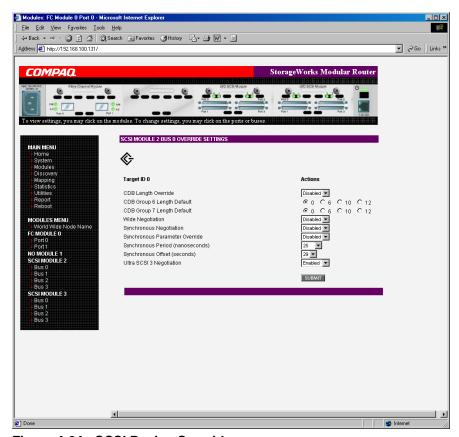
Figure 4-24: SCSI Device Override screen
