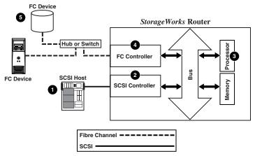
Figure 1-11: Converting SCSI to Fibre Channel Protocol Process
