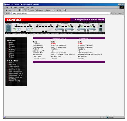
Figure 4-17: Fibre Channel module status screen
