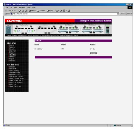
Figure 4-33: Beacon configuration screen
