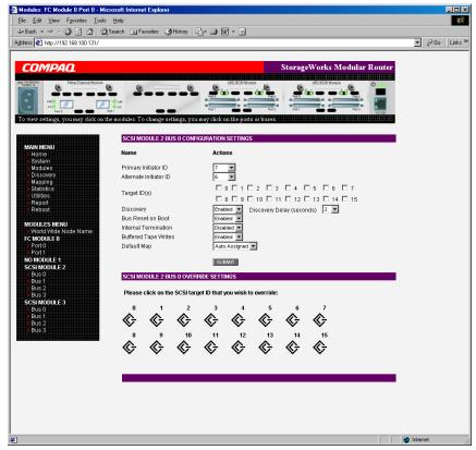
Figure 4-23: SCSI Module Bus Configuration Settings screen
