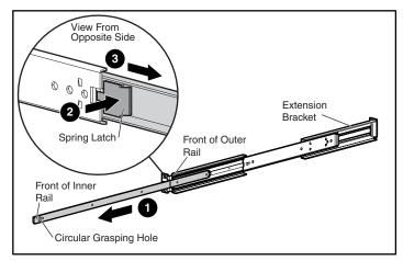
Figure 2-1: Separating the inner and outer rails
