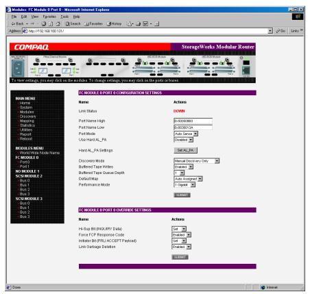
Figure 4-19: Fibre Channel module port configuration settings screen
