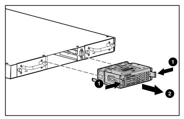
Figure 7-4: Removing the fan module
