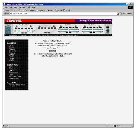
Figure 4-14: Reset to Factory Default screen
