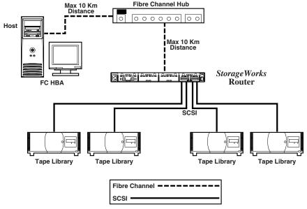
Figure 2-9: Configuration with tape library using Arbitrated (or Private) loop
