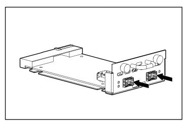
Figure 2-10: Fibre Channel ports
