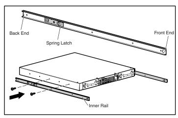
Figure 2-3: Attaching inner rails to the router
