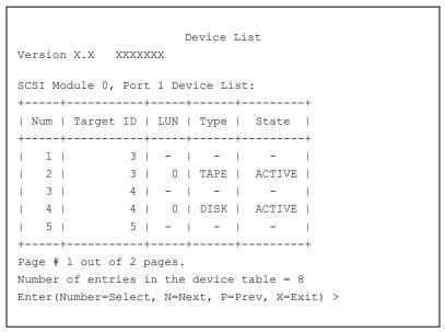
Figure 5-20: Device List generated for a SCSI port
