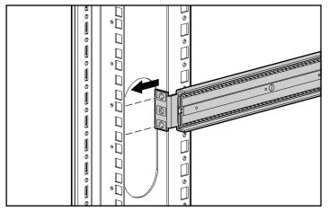
Figure 2-2: Aligning the bracket face with the rack
