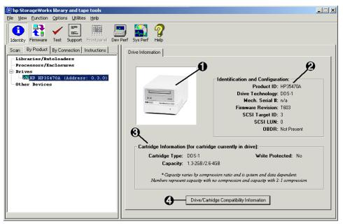
Figure 3: Device Information screen showing a standalone device
