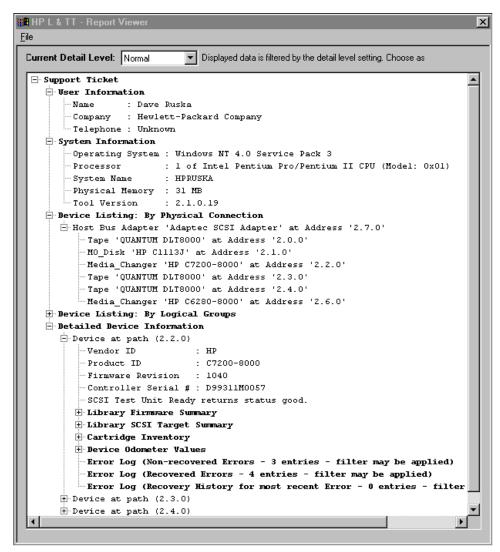
Figure 15: Example support ticket with normal detail (Windows version)
