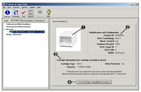
Figure 3: Device Information screen showing a standalone device
