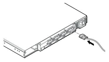
Figure 2-4. Connecting the serial cable
