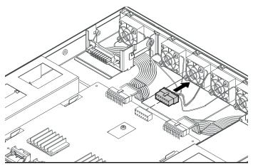
Figure 6-6. Disconnecting the wiring harness
