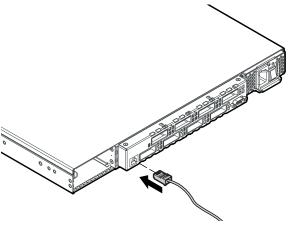
Figure 2-5. Connecting the Ethernet cable
