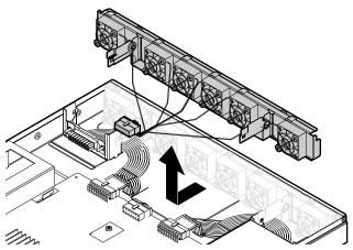
Figure 6-7. Removing the fan assembly
