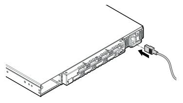
Figure 2-3. Connecting the power cord
