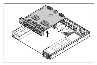
Figure 6-10. Removing the motherboard
