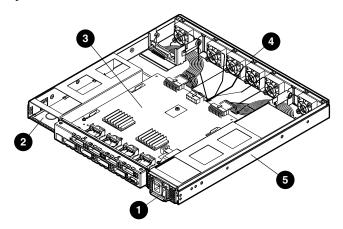
Figure 6-1. Switch components
