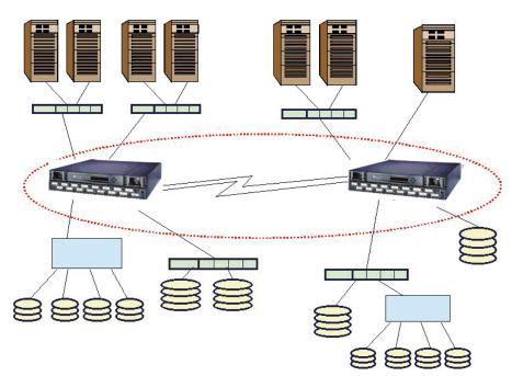
Figure 6-6: QuickLoop configured as a dual switch
