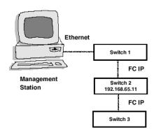
Figure 5-2: Single-port management of switches
