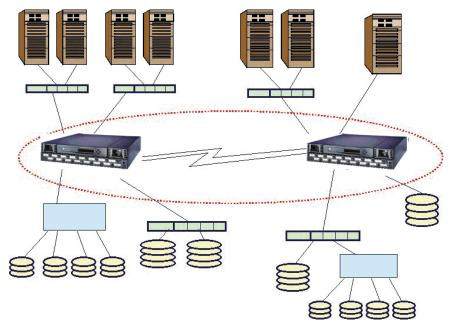
Figure 6-7: QuickLoop configured as a long-distance QuickLoop
