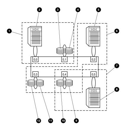
Figure 6-9: Port-based QuickLoop Zoning example
