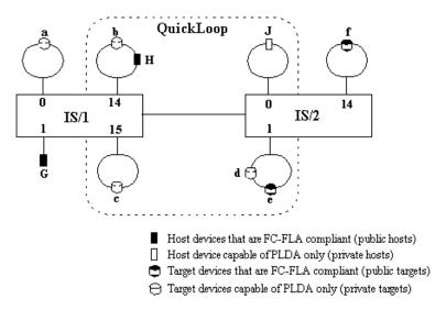
Figure 6-8: QuickLoop configuration in mixed mode
