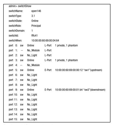
Figure A-82: switchShow command example
