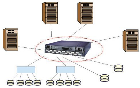
Figure 6-5: QuickLoop-enabled switch used as a concentrator
