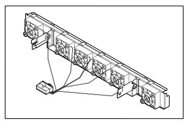
Figure 6-4. Fan assembly
