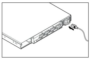
Figure 2-3. Connecting the power cable
