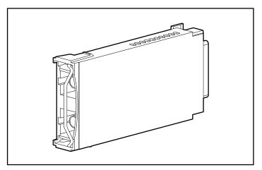
Figure 6-2. GBIC module with a locking bar
