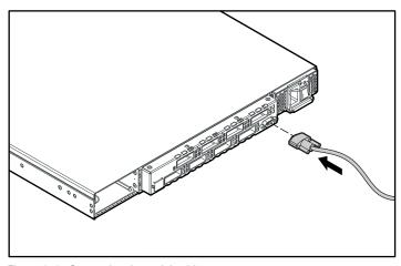
Figure 2-4. Connecting the serial cable
