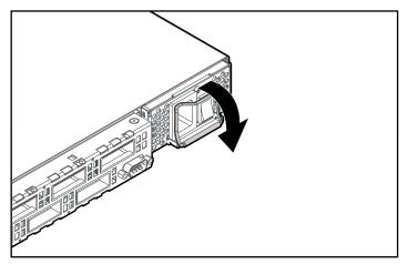
Figure 6-1. Metal handle on the power supply
