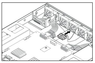
Figure 6-5. Disconnecting the wiring harness
