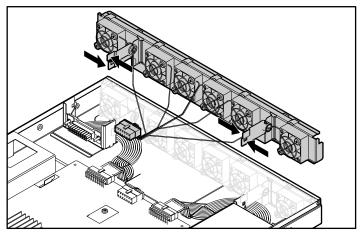
Figure 6-7. Releasing the tabs on the fan assembly
