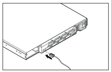
Figure 2-5. Connecting the Ethernet cable
