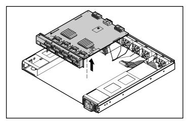
Figure 6-9. Removing the motherboard
