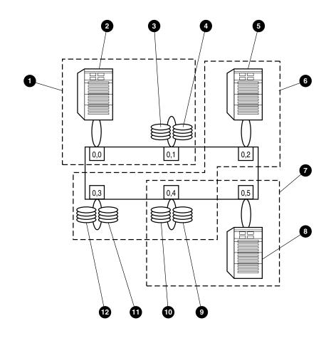
In Figure 5-3, three QuickLoop zones have been defined. The notation is <switch #, port #>.
