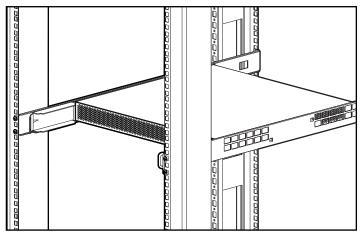
Figure 2-7. Hub loaded in the rack
