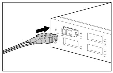
Figure 2-15. Installing a Fibre Channel cable
