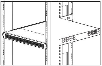
After the hub is installed in the rack, you are ready to connect the Multi-Mode Fibre Channel Cables and to power up the unit.
