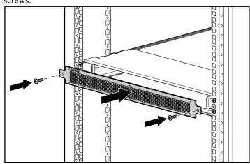
5. Install the 1U faceplate with two M6 x 1.0-12L Phillips screws.
