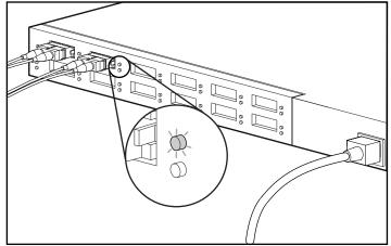
Figure 3-2. Checking the GBIC LEDs
