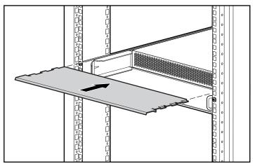
Figure 2-9. Installing the top air baffle
