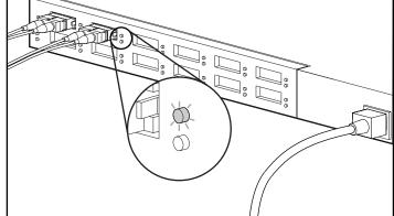
Figure 2-17. Checking the GBIC LEDs
