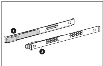
Figure 2-3. Chassis slide rail ① and the rack mounting rail ②
