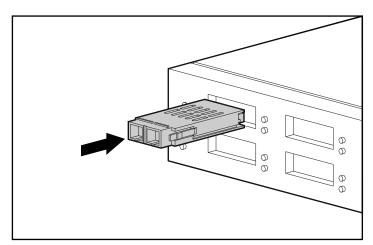
Figure 2-14. Installing a GBIC module
