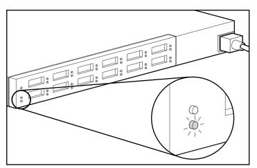
Figure 3-1. Checking the power LED and the fault LED
