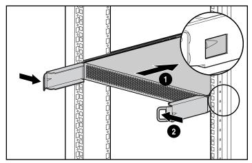
Figure 2-6. Loading the Hub in the rack
