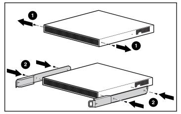
Figure 2-5. Attaching chassis slide rails
