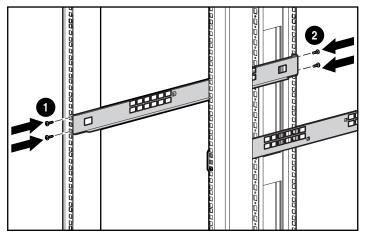
Figure 2-4. Installing the rack rails
