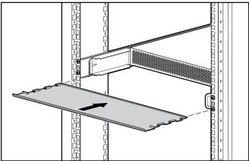
Figure 2-8. Installing the bottom air baffle
