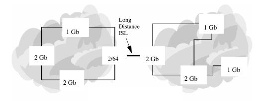
Figure 3–3: Mixed Extended Fabric with Core Switch 2/64 to StorageWorks 2 Gb SAN switch ISL long distance port switches
