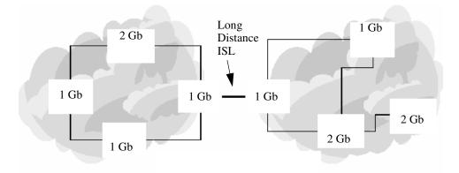
Figure 3–1: Mixed Extended Fabric with StorageWorks 1 Gb SAN switch series ISL long distance port switches
