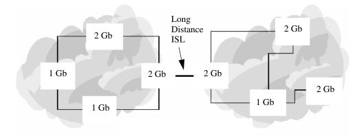
Figure 3–2: Mixed Extended Fabric with StorageWorks 2 Gb SAN switch series ISL long distance port switches
