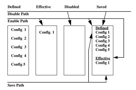
Figure 3–1: Enabling a zone configuration
