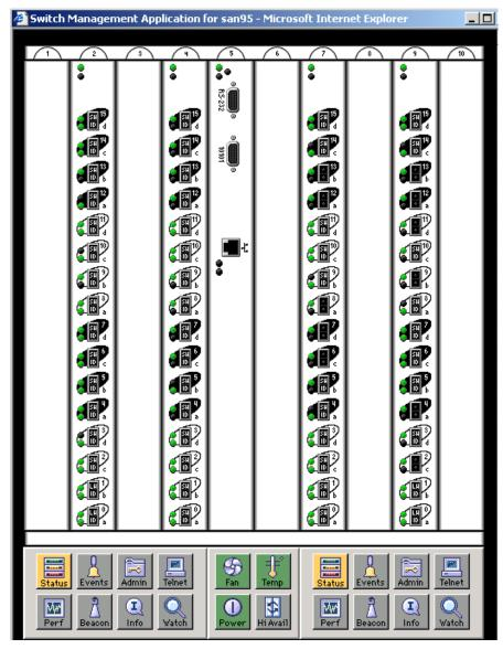
Figure 1-2: Switch View of StorageWorks Core switch series switch
