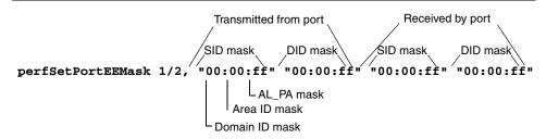
Figure 14: Mask positions for end-to-end monitors
