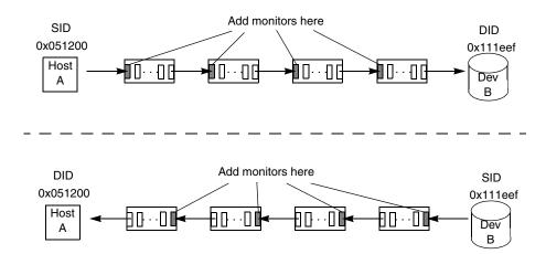
Figure 13: Proper placement of end-to-end performance monitors
