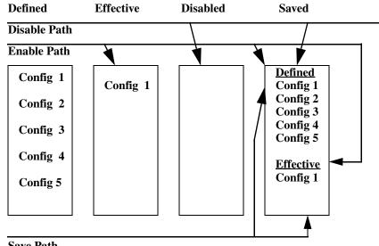
In Figure 2, the defined and effective configurations are saved to flash:
