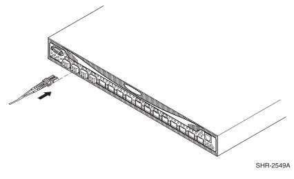
Figure 17: Inserting a cable into an SFP
