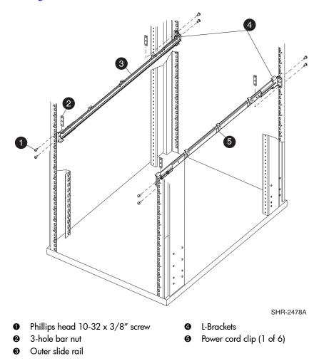
Figure 6: Attaching the outer slide rails to the HP 9000 Series rack
