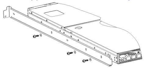
Figure 12: Assembling the inner rails
