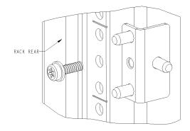
Figure 8: Installing the mounting brackets
