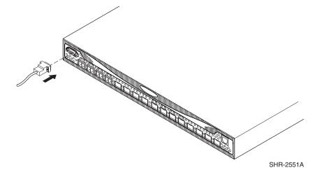
Figure 15: Connecting the Serial cable
