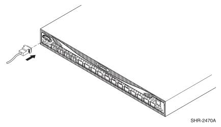
Figure 2–7: Connecting the Serial cable
