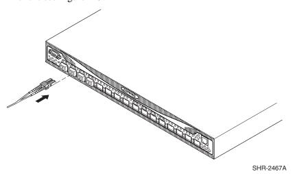
Figure 2-9: Installing an SFP
