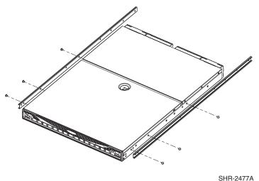
Figure 2-2: Securing the Inner Slide Rails to the switch
