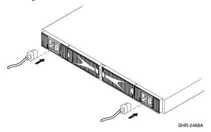
Figure 2-6: Connecting the power cords
