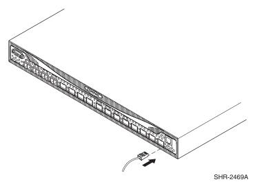
Figure 2-8: Connecting the Ethernet Cable
