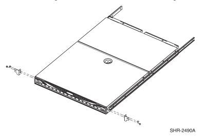
Figure 2-3: Attaching the Rear Rack Mount Brackets
