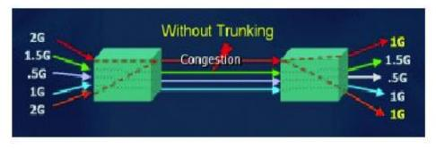
Figure 1–1: Routing without the ISL Trunking Feature
