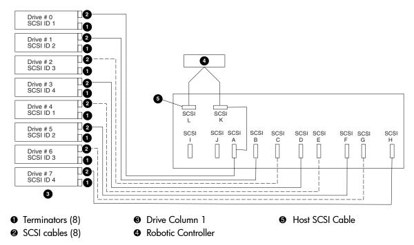
Figure 12: Internal SCSI cabling configuration (ESL9322)
