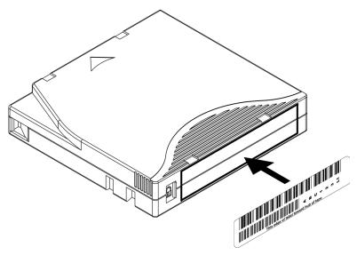
Figure 16: Attaching an Ultrium bar code label
