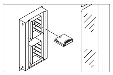
Figure 21: Inserting a tape cartridge into a magazine
