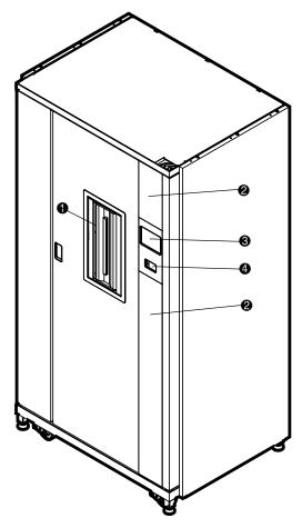
Figure 1: Cabinet front panel (ESL9322)
