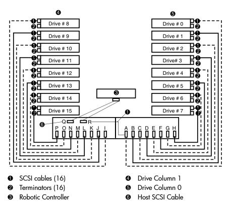
Figure 14: Internal SCSI cabling configuration (ESL9595)
