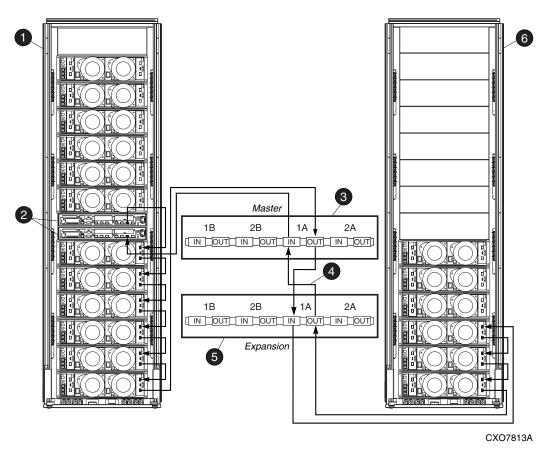
Figure 1-5: Configuration 2C12D + 0C6D—Fibre Channel Loop 1A
