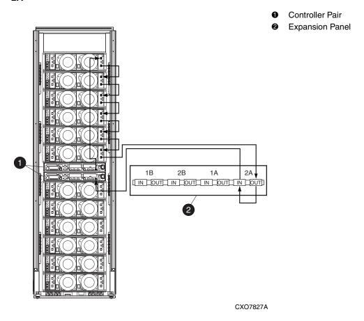
Fibre Channel Loop 2B is located on the upper left side of the rack (viewed from the rear). Loop 2B is one continuous loop that connects the M5214 drive enclosures to the controller pair. Figure 1–20 shows Fibre Channel Loop 2B.
