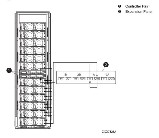
Fibre Channel Loop 1B is located on the lower left side of the rack (viewed from the rear). Loop 1B is one continuous loop that connects the M5214 drive enclosures to the controller pair. Figure 1–18 shows Fibre Channel Loop 1B.
