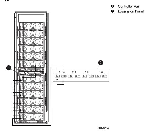
Fibre Channel Loop 2A is located on the upper right side of the rack (viewed from the rear). Loop 2A is one continuous loop that connects the M5214 drive enclosures to the controller pair. Figure 1–19 shows Fibre Channel Loop 2A.
