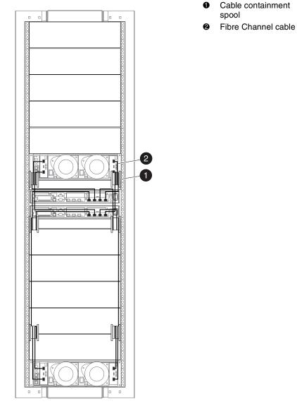
Figure 1–7 shows the cable management configuration for the 2C2D configuration.
