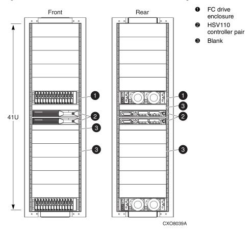
Figure 1–1 shows the front and rear views of the 2C2D configuration.
