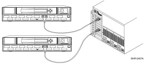
Figure 3: Cabling hosts to switches
