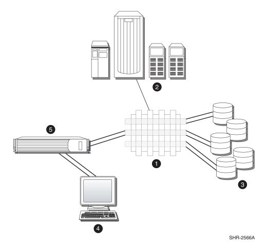
Figure 1: SAN architecture for single path
