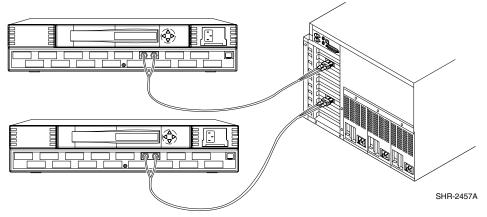
Figure 2: Cabling hosts to switches
