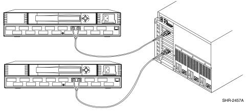
Figure 2: Cabling hosts to switches
