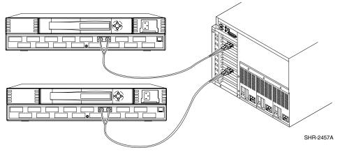
Figure 2: Cabling hosts to switches
