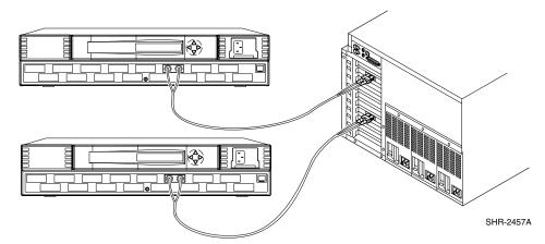
Figure 4-2: Cabling Hosts to Switches
