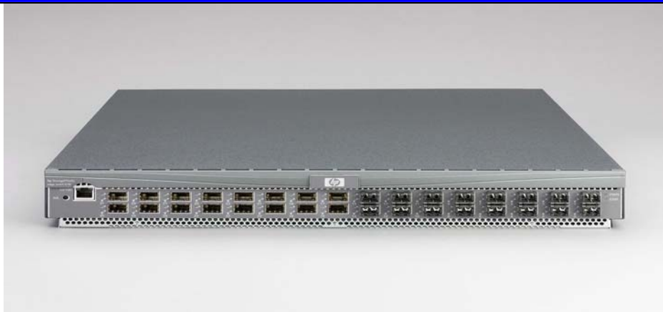
Edge switch 2/32 Front view (32 ports, 16 enabled, SFP's installed)
