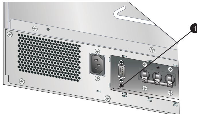
Figure 4-2: ESD Grounding Point (Rear)
