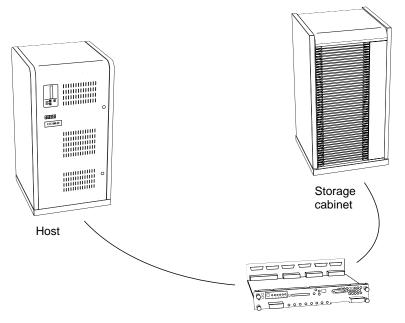
From the subsystem's perspective, the controller receives the I/O requests from the host and directs them to the devices in the subsystem. Since the controller processes all of the I/O requests, it eliminates the host-based processing that's typically associated with reading and writing data to multiple storage devices.
