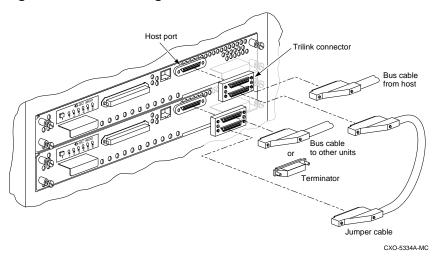
To connect a pair of dual-redundant controllers to the host:
