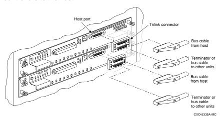
To connect a pair of multiple bus failover dual-redundant controllers to the host:
