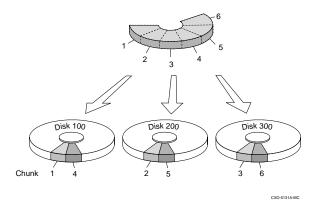
The relationship between the chunk size and the average request size determines if striping maximizes the request rate or the data-transfer rate. You can set the chunk size or let the controller set it automatically. See *Chunk size* on page 3–18 for information about setting the chunk size.
