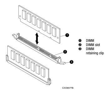
Figure 4. Removing or installing a DIMM
