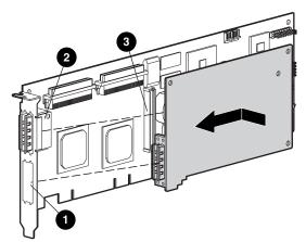
2. Plug the adapter board into the connector ③ on the array controller board.
