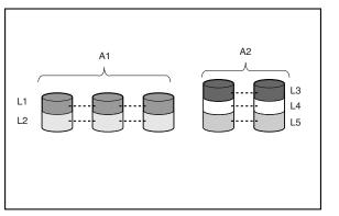
Figure 3-5: Two arrays (A1, A2) and five logical drives (L1 through L5) spread over five physical drives
