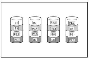
Figure 3-8: RAID ADG (advanced data guarding) with two sets of parity data
