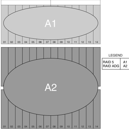
Figure 4-3: Horizontal Array configurations
