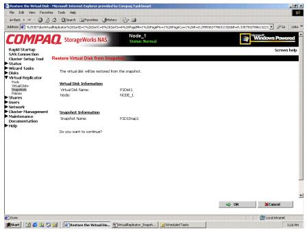
Figure 6-26: Restore Virtual Disk from Snapshot screen
