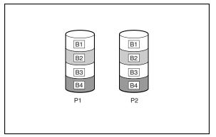
Figure 3-6: RAID 1 (drive mirroring) of P1 onto P2
