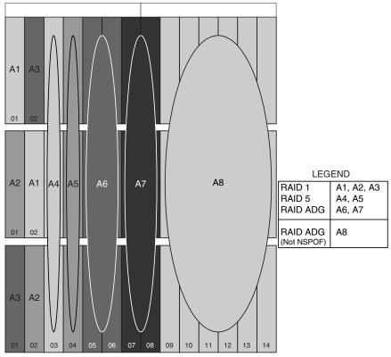
Figure 4-2: Vertical Array configurations
