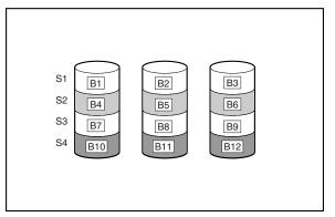
Figure 3-4: RAID 0 (data striping) (S1-S4) of data blocks (B1-B12)
