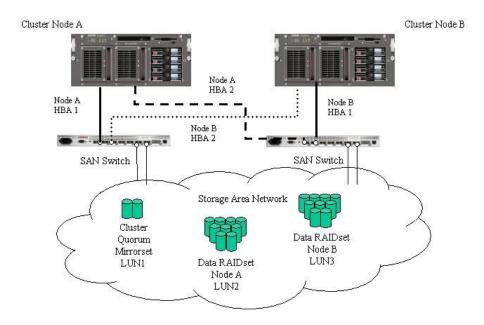
Figure 11-1: NAS B3000 cluster diagram
