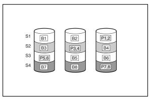
Figure 3-7: RAID 5 (distributed data guarding) showing parity information (P)
