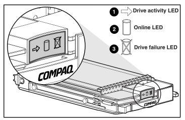
Figure 5-1: Hot-plug hard drive LED indicators
