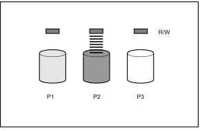
Figure 3-2: Separate physical drive (P1, P2, P3) read/write (R/W) operations
