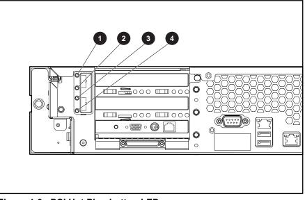
Figure 4-6: PCI Hot Plug button LEDs
