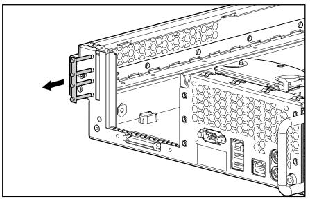
Figure 2-38: Sliding the lightpipe out of the chassis
