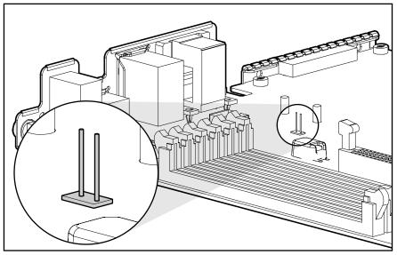
The NAS B2000 contains one two-pin bootblock flash jumper. It enables the user to configure the system board for a bootblock flash of the system ROM (Figure 4-14).
