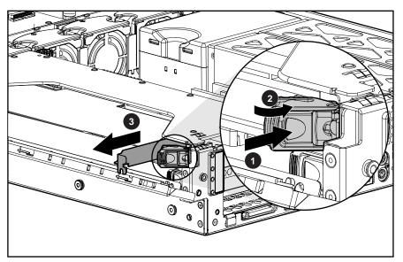
Figure 2-17: Removing the expansion slot cover from slot 3
