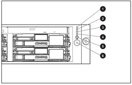
The five LEDs on the front of the device indicate device status. Figure 4-3 and Table 4-3 identify and describe the LED locations and functions.
