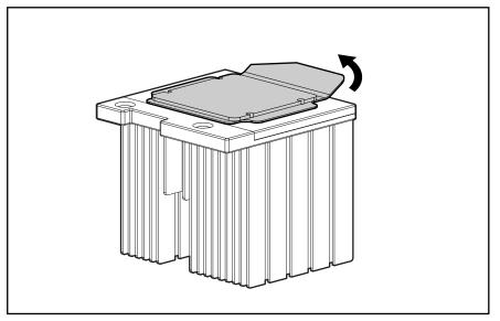
Figure 2-46: Removing the plastic strip on the heatsink
