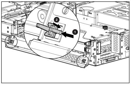
Figure 2-15: Removing the PCI riser cage door latch
