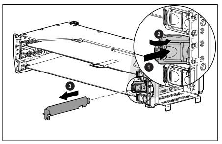
Figure 2-33: Removing the expansion slot cover
