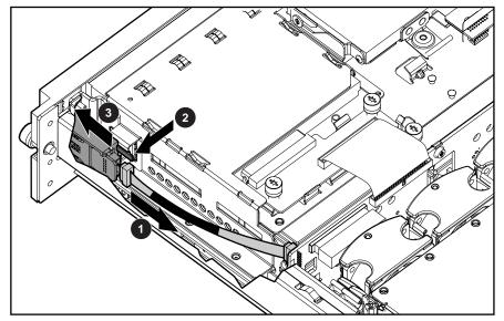
Figure 2-41: Removing the power button/LED board
