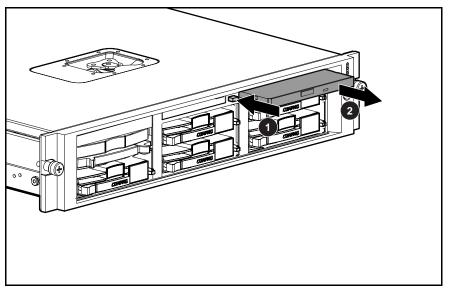
Figure 2-22: Ejecting the CD-ROM drive
