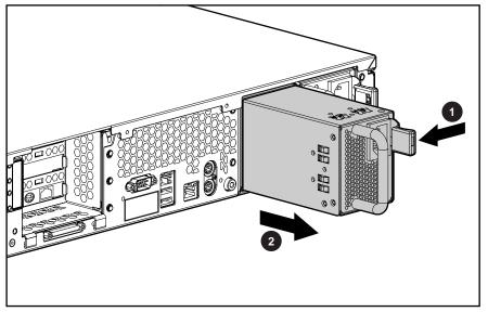
Figure 2-8: Removing a hot-plug power supply
