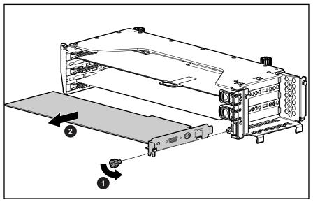
Figure 2-32: Removing a Remote Insight Lights-Out Edition board
