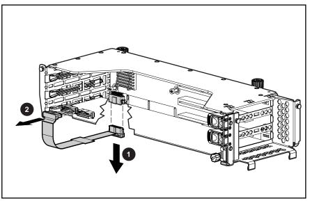
Figure 2-31: Removing the Remote Insight Lights-Out Edition board interface cable (PCI expansion board ejector/divider removed for clarity)
