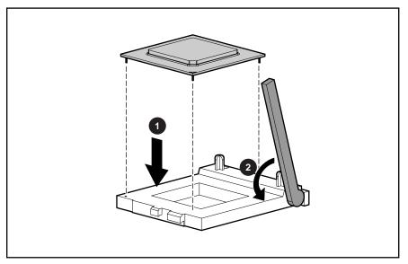
Figure 2-45: Installing the processor
