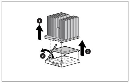
Figure 2-44: Removing the heatsink and processor from the system board
