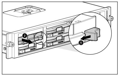
Figure 2-5: Removing a hard drive blank
