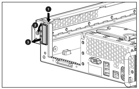
Figure 2-37: Removing the PCI lightpipe cover
