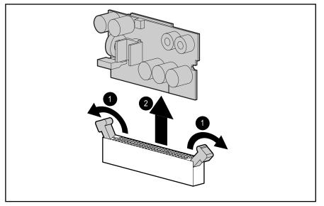
Figure 2-48: Removing a PPM
