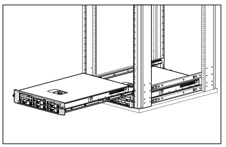
Figure 2-1: Extending the device from the rack
