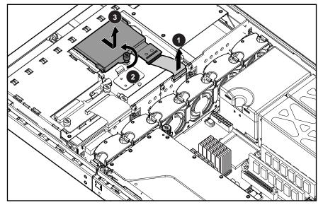
Figure 2-23: Removing the diskette drive
