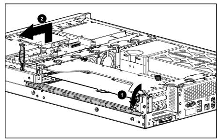
Figure 2-13: Removing the PCI shipping bracket
