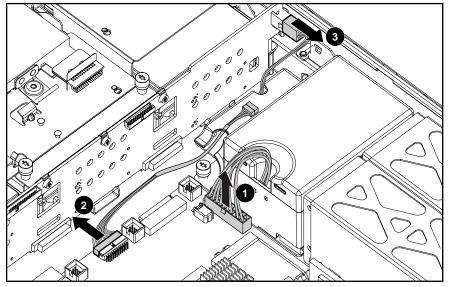
Figure 2-39: Disconnecting the power cables
