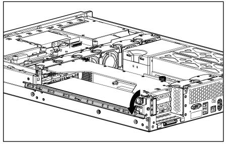
Figure 2-18: Opening the PCI riser cage door
