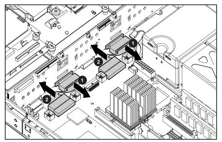
Figure 2-58: Removing the system cables (PCI riser cage removed for clarity)
