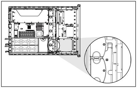
Figure 4-11: Power converter module LED
