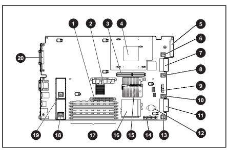
Figure 4-2 and Table 4-2 show the connectors on the system board.
