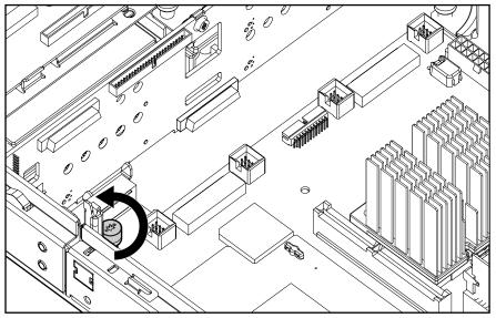
Figure 2-51: Loosening the system board thumbscrew
