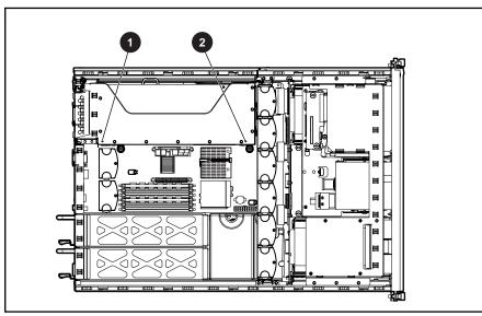
Figure 4-5: PCI riser cage LEDs
