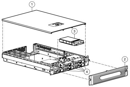
Figure 1-1: Exploded view of the StorageWorks NAS B2000 mechanical parts
