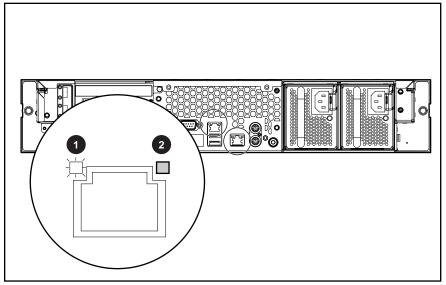
Figure 4-7: RJ-45 network connector LEDs
