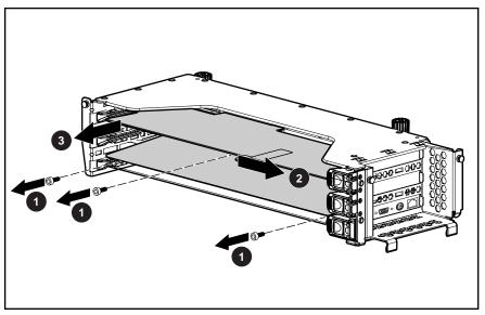
Figure 2-34: Removing the PCI expansion board ejector/divider
