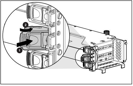
Figure 2-35: Opening the PCI slot release lever
