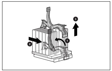
Figure 2-43: Disengaging the heatsink-retaining clip
