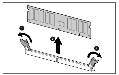
Figure 2-42: Removing a DIMM
