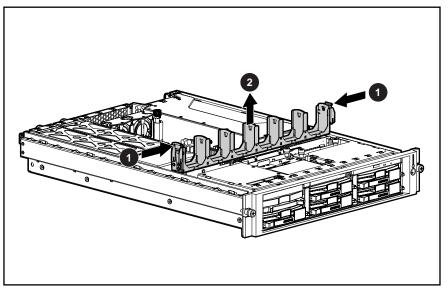
Figure 2-27: Removing the front fan bracket
