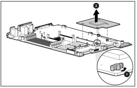
Figure 2-49: Removing the Smart Array 5i Controller
