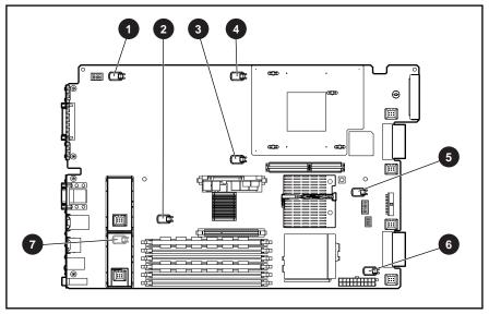
Figure 2-52: Identifying the alignment keys and keyhole locations
