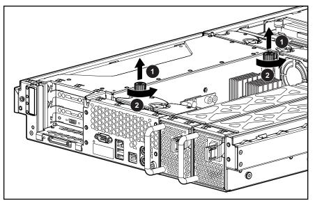
Figure 2-29: Loosening the PCI riser cage thumbscrews
