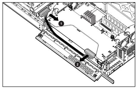
Figure 2-60: Removing the long SCSI cable
