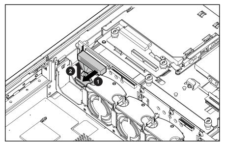
Figure 2-55: Removing the short SCSI cable (PCI riser cage and fan removed for clarity)
