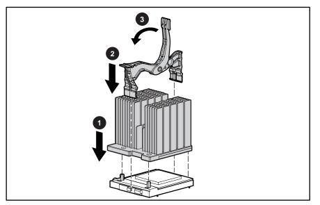
Figure 2-47: Installing the heatsink and heatsink-retaining clip
