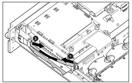
Figure 2-57: Removing the power button/LED cable
