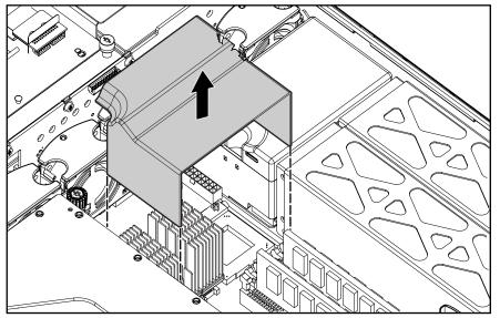
Figure 2-12: Removing the air baffle
