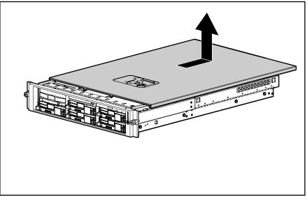
4. Slide the access panel toward the rear of the unit about 1.25 cm (0.5 inch) and lift to remove the panel.
