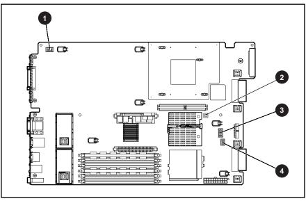
Figure 4-13: System board switches
