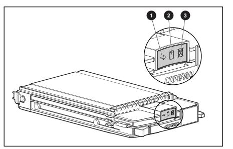
Figure 4-4: Hot-plug SCSI hard drive LEDs
