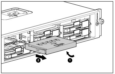
Figure 2-6: Removing the tape drive blank
