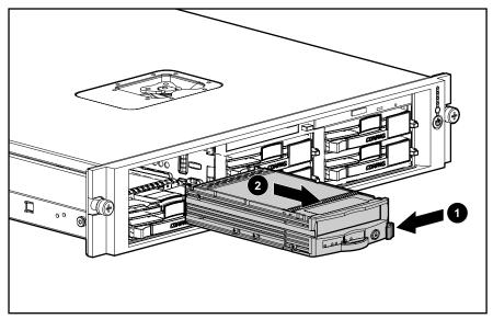
Figure 2-7: Removing a universal hot-plug tape drive
