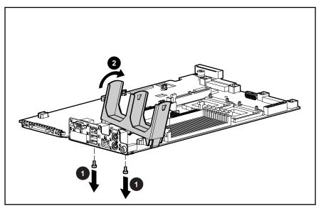
Figure 2-54: Removing the rear fan bracket
