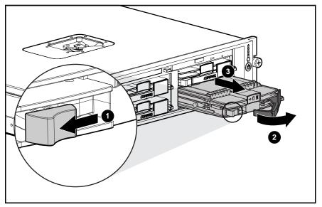
Figure 2-4: Removing a hot-plug SCSI hard drive
