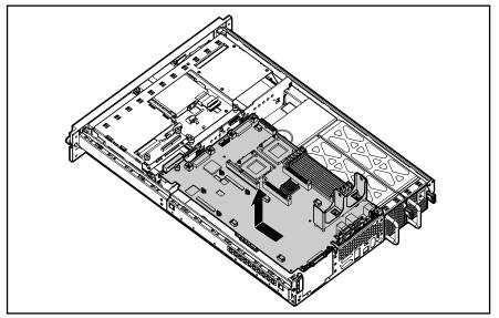
Figure 2-53: Removing the system board from the chassis
