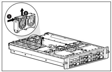
Figure 2-11: Removing a fan
