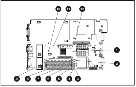
Figure 4-12: System board LEDs
