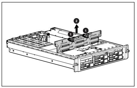
Figure 2-28: Removing the SCSI backplane
