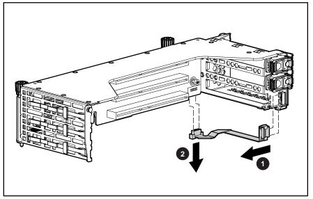
Figure 2-59: Removing the PCI Hot Plug backplane cable (PCI expansion board ejector/divider removed for clarity)
