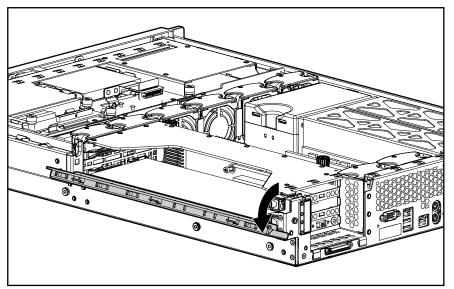
Figure 2-14: Opening the PCI riser cage door
