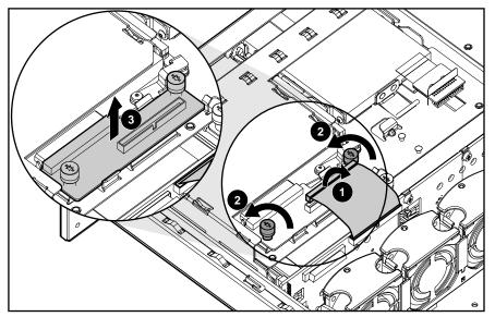
Figure 2-24: Removing the CD MultiBay adapter board
