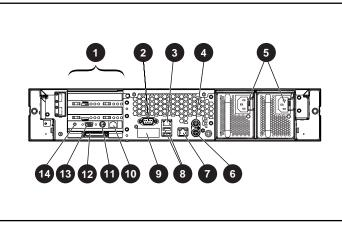
Figure 4-1: Rear panel connectors
