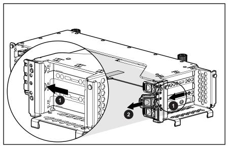
Figure 2-36: Removing the PCI slot release lever
