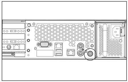
Figure 4-8: Rear unit identification LED switch
