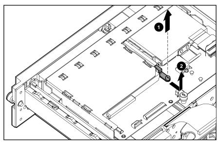
Figure 2-26: Removing the CD ejector assembly
