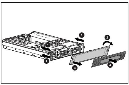
Figure 2-21: Removing the front bezel and faceplate
