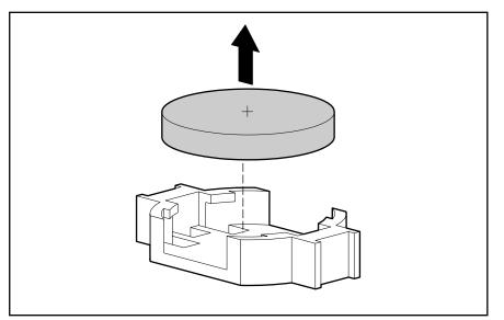
Figure 2-50: Removing the battery
