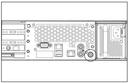
Figure 2-3: Rear unit identification LED switch
