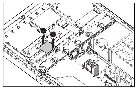
Figure 2-56: Removing the CD MultiBay cable
