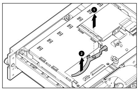
Figure 2-25: Removing the ejector lever
