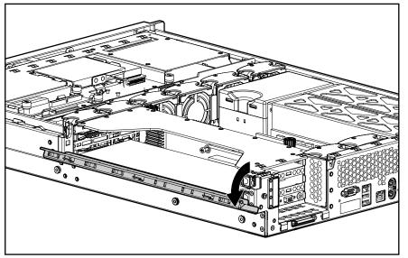
Figure 2-16: Opening the PCI riser cage door
