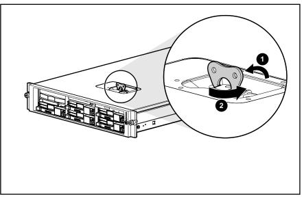
Figure 2-9: Unlocking the hood latch
