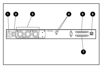
Power supply connector **2** Power switch
