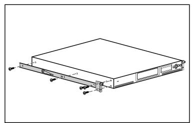
1. Install an inner rail to the side of the AutoLoader using the provided screws, as shown.
