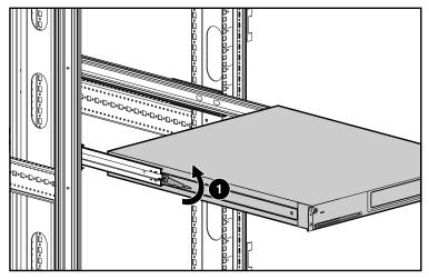
**IMPORTANT:** Do not unlock the mounting rails while sliding the AutoLoader into place. The rails will unlock automatically as the AutoLoader is slid into position.
