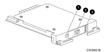
Figure 1–10. BA370 enclosure PVA module connector and switches
