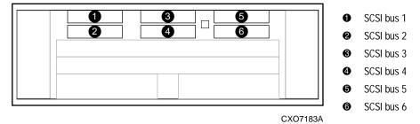
Figure 4–11. I/O module bay to SCSI bus number correlation
