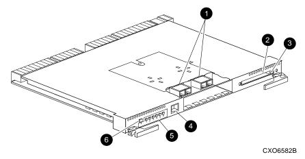
Figure 1-6. HSG80 array controller front panel connectors, switches, and LEDs
