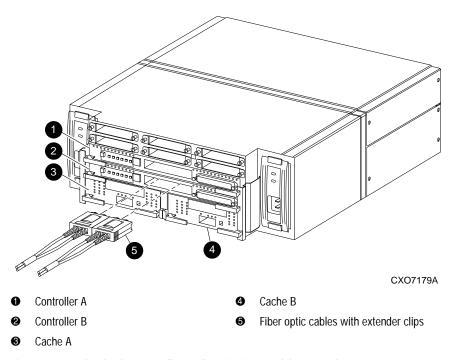
Figure 4–6. Dual-redundant controller configuration in a Model 2200 enclosure
