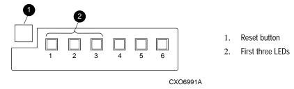
Figure 3-1. Controller reset button and first three LEDs
