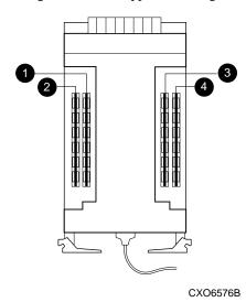
Figure 2–7. Cache module DIMM locations
