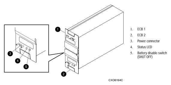
Figure 3–2. ECB battery disable switch location (dual ECB example)
