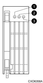
Figure 1–13. Model 2200 enclosure ECB LEDs
