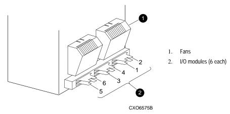
Figure 3-10. I/O module locations in a BA370 enclosure
