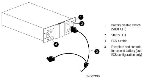
Figure 3–8. Dual ECB configuration
