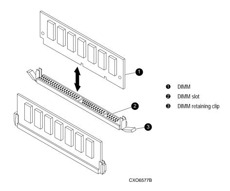
Figure 2–8. DIMM components
