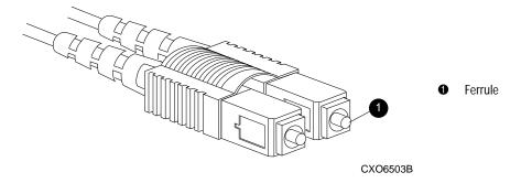
Figure 2-2. Ferrule on a fiber optic cable
