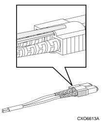
Figure 2–6. Using thin needle-nose pliers to disconnect a fiber optic cable
