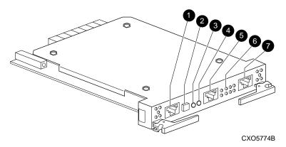
Figure 1–11. BA370 enclosure EMU connectors, switches, and LEDs
