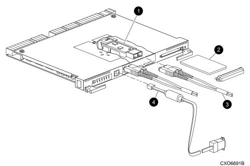
Figure 1–4. HSG80 array controller—GLM, cabling, and program card
