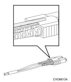
Figure 3–4. Using thin needle-nose pliers to disconnect a fiber optic cable
