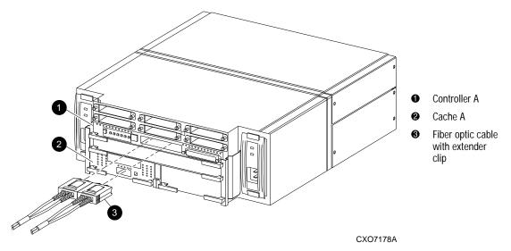
Figure 4-2. Single-controller configuration in a Model 2200 enclosure
