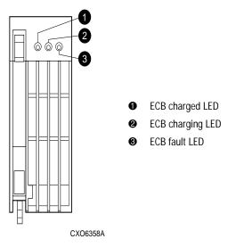
Figure 4–9. ECB status LEDs
