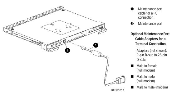
Figure 2–1. PC/terminal to maintenance port connection
