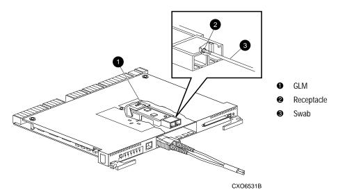
Figure 2-3. Cleaning procedure for GLM
