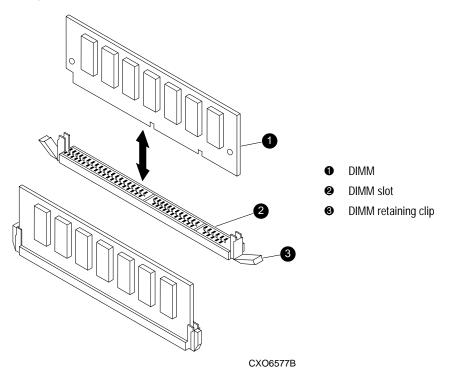
Figure 4–5. DIMM components
