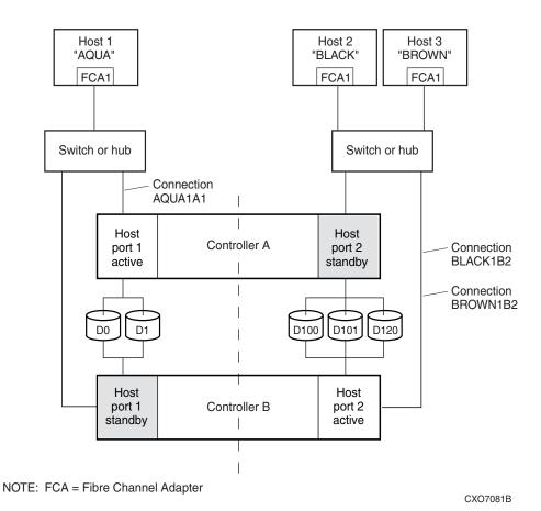
Figure 1–9: Connections in separate-link, transparent failover mode configurations
