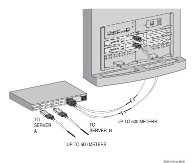
Figure C-2: Cable Connection—Storage RAID Array to Fibre Channel switch
