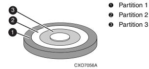
Figure 2–12: One example of a partitioned single-disk unit
