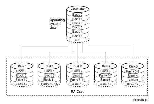
Figure 2-9: 5-member RAIDset using parity
