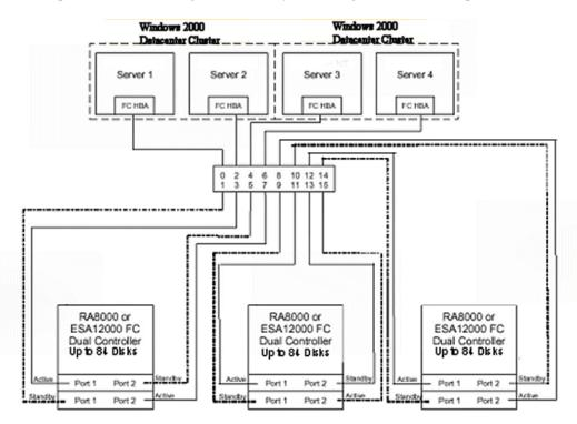
Figure C-3: Two Windows 2000 Datacenter clusters—Fibre Channel switch
