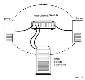
Figure C-1: Storage RAID Array Fibre Channel cluster concept
