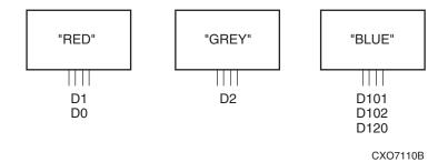
Figure 6-3: Example, logical or virtual disks comprised of storagesets
