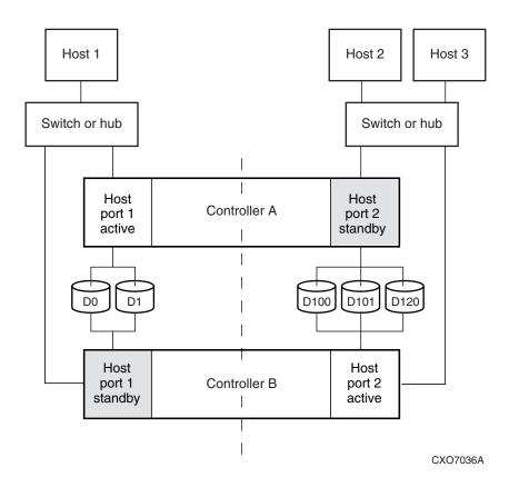
Figure 1-5: Transparent failover—normal operation
