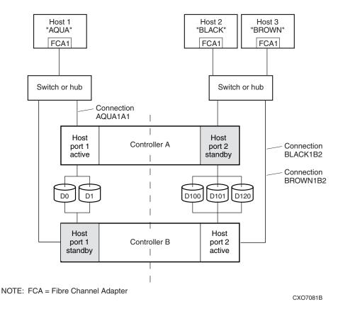
Figure 1–11: Limiting host access in transparent failover mode
