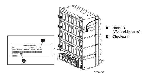
Figure 1-14: Placement of the worldwide name label on the BA370 enclosure
