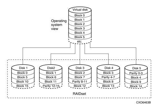
Figure 2-9: 5-member RAIDset using parity
