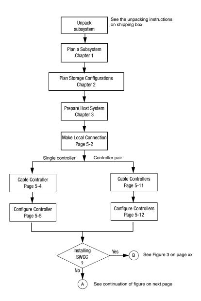
Figure 1: General configuration flowchart (panel 1)
