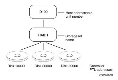
Figure 2-1: Mapping a unit to physical disk drives
