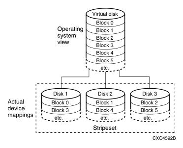
Figure 2–3: How data is laid out on disks in BA370 enclosure configuration
