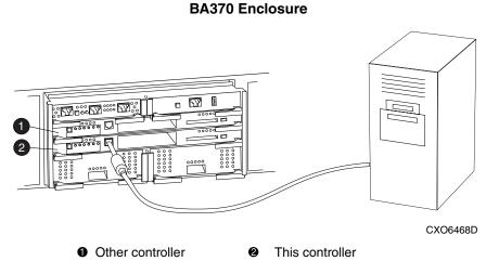
Figure 1-4: "This controller" and "other controller" for the BA370 enclosure
