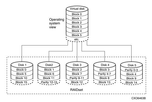
Figure 2-9: 5-member RAIDset using parity
