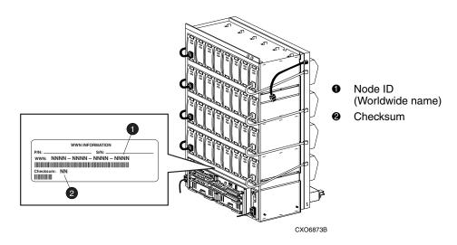
Figure 1-10: Placement of the worldwide name label on the BA370 enclosure
