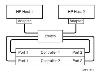
Figure 3-3. Single switch HP MC/ServiceGuard cluster, high availability configuration
