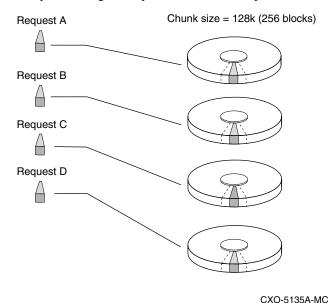
Figure 2-18. Chunk size larger than the request size
