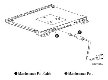
Figure 5–1. Maintenance port connection
