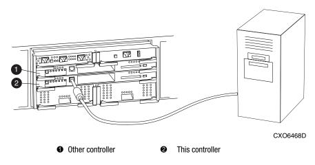
Figure 1-4. "This controller" and "other controller" for the BA370 enclosure
