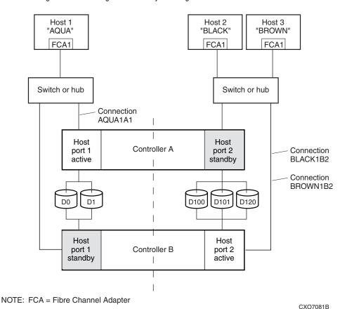
Figure 1–13. Limiting host access in transparent failover mode
