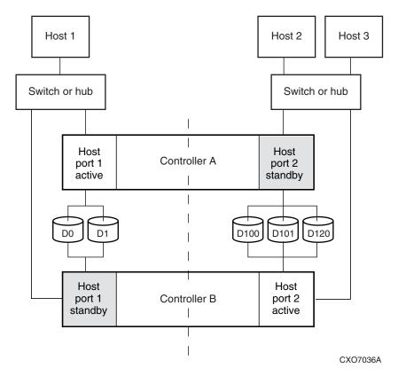
Figure 1–5. Transparent failover—normal operation
