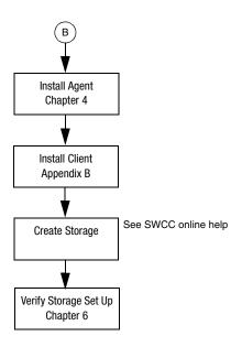
Figure 3. Configuring storage with SWCC
