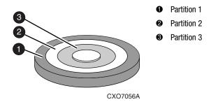
Figure 2-17. One example of a partitioned single-disk unit
