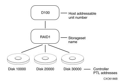
Figure 2-7. Mapping a unit to physical disk drives
