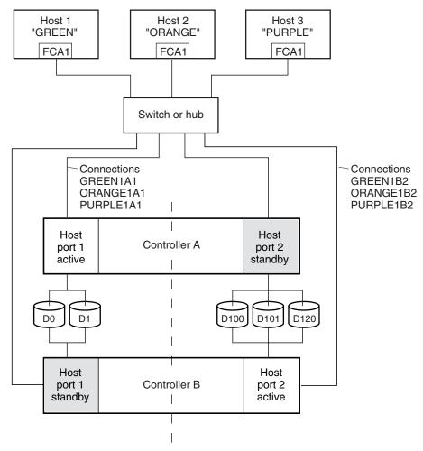
NOTE: FCA = Fibre Channel Adapter
