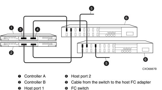
Figure 5–3 shows a controller pair with failover cabling showing one HBA per server with HSG80 controller in transparent failover mode.
