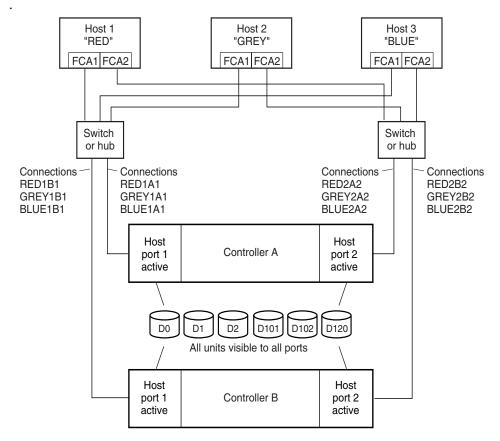
NOTE: FCA = Fibre Channel Adapter
