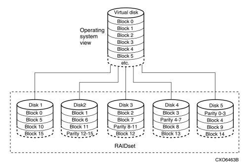
Figure 2–9: 5-member RAIDset using parity
