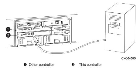
Figure 1-4: "This controller" and "other controller" for the BA370 enclosure
