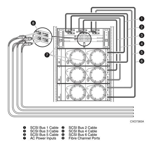
Figure 3–1: Dual-Bus Enterprise Storage RAID Array Storage System
