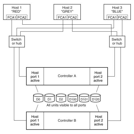
NOTE: FCA = Fibre Channel Adapter
