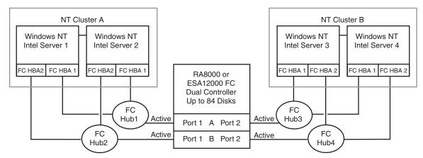
Figure C-6: Two-Cluster Fibre Channel Configuration with Secure Path
