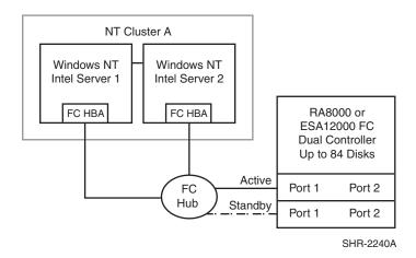
Figure C-3: Single Cluster Fibre Channel Configuration
