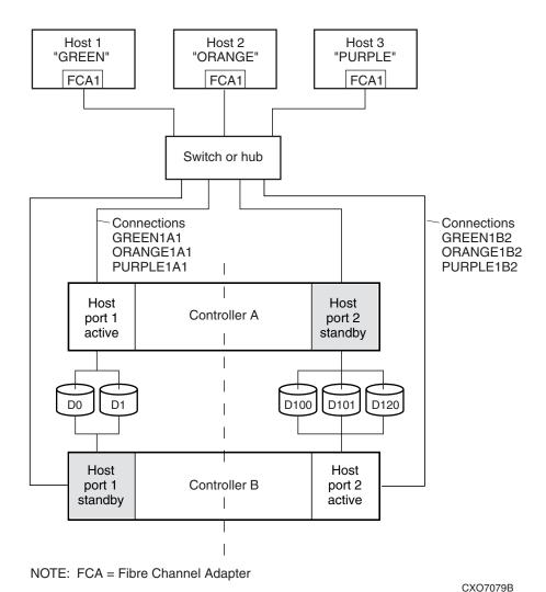
Figure 1–10: Connections in single-link, transparent failover mode configurations
