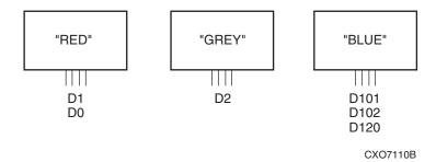
Figure 6–4: Example, logical or virtual disks comprised of storagesets
