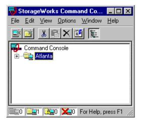
Figure B-2: Navigation window showing storage host system "Atlanta"
