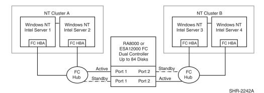
Figure C-5: Two-Cluster Fibre Channel Configuration
