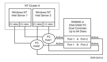
Figure C-4: Single Cluster Fibre Channel Configuration with Secure Path
