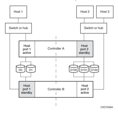
Figure 1–5: Transparent failover—normal operation
