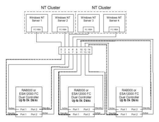
Figure C-7: Two Windows NT/Windows 2000 Clusters - Fibre Channel Switch
