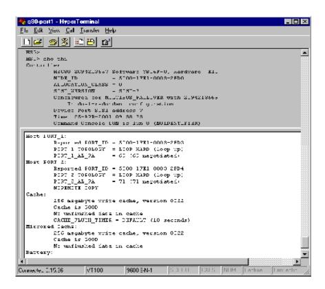
Figure C-21: Verifying FC-AL Connectivity RAID Array Subsystem
