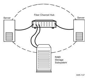
Figure C-1: Storage RAID Array Fibre Channel Cluster Concept
