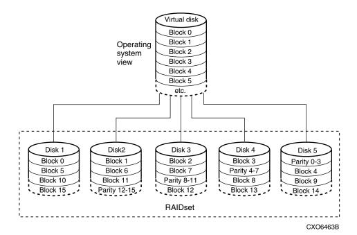
Figure 2–9: 5-member RAIDset using parity
