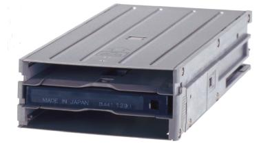
Figure 2: Autoloader eight-tape cassette magazine
