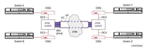
Figure 5 ATM inverse multiplexing configuration
