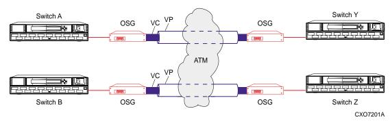
Figure 2 Dual-link configuration
