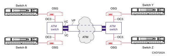
Figure 3 Shared virtual channel link configuration
