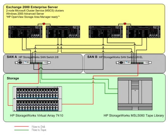
figure 2 - example mid-market Exchange solution physical view
