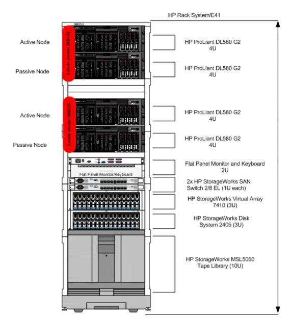
figure 3 - example mid-market Exchange solution rack
